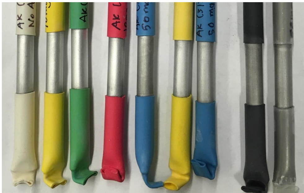
Figure 11. Samples after corrosion testing. The average mass lost was 0.05g, ranging from 0.02 to 0.07g. From left to right: no additives, 10mg mellitic acid, 50mg mellitic acid, 10mg trimesic acid, 50mg trimesic acid, 10mg citric acid, 50mg citric acid, 10mg EDTA, 50mg EDTA.
