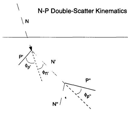
Figure 1: Schematic of non-relativistic double scatter neutron event in a block of plastic scintillator.
