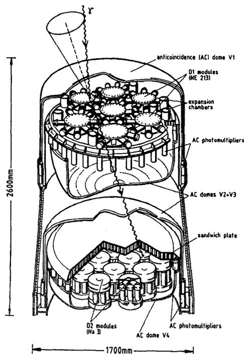
Fig. 1: Schematic diagram of COMPTEL
