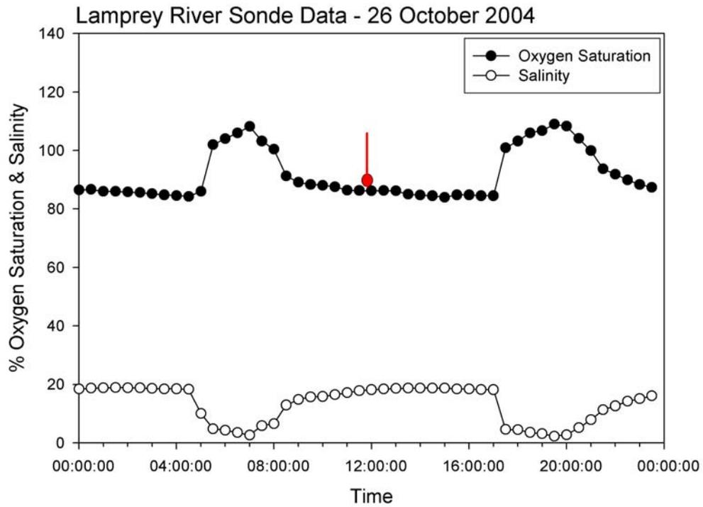
**Figure 5 –Oxygen Saturation (solid dots) and Salinity (open dots) data from the Lamprey River DataSonde on 26 October. Red dots (DataSonde depth) and line (range) for vertical casts taken adjacent to the DataSonde during spatial survey on the same date.**
