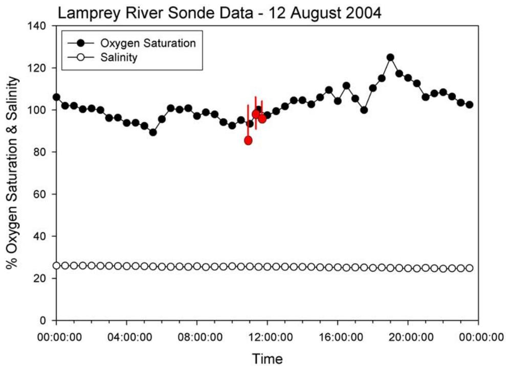
**Figure 4 –Oxygen Saturation (solid dots) and Salinity (open dots) data from the Lamprey River DataSonde on 12 August. Red dots (DataSonde depth) and line (range) for vertical casts taken adjacent to the DataSonde during spatial survey on the same date.**
