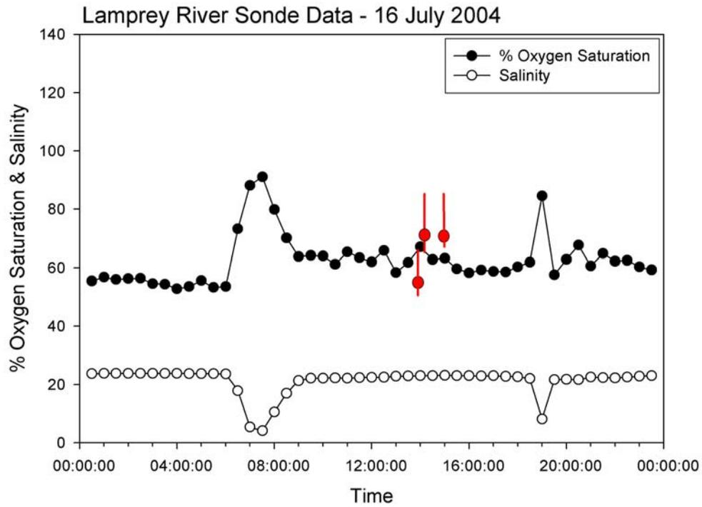
**Figure 2 –Oxygen Saturation (solid dots) and Salinity (open dots) data from the Lamprey River DataSonde on 16 July. Red dots (DataSonde depth) and line (range) for vertical casts taken adjacent to the DataSonde during spatial survey on the same date.**
