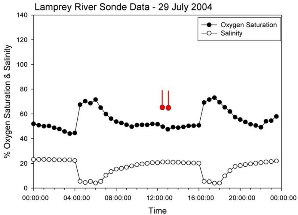
**Figure 3 –Oxygen Saturation (solid dots) and Salinity (open dots) data from the Lamprey River DataSonde on 29 July. Red dots (DataSonde depth) and line (range) for vertical casts taken adjacent to the DataSonde during spatial survey on the same date.**
