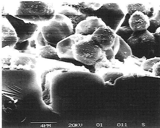
Figure 3. A view shown for comparison of standard granular commercial Gd<sub>2</sub>O<sub>2</sub>S deposited on the same fiberoptic substrate. The irregular structure and poor packing fraction of standard phosphor screen material compared to our CsI films can be clearly seen.
