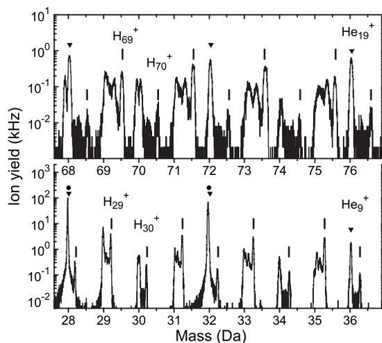
FIG. 2. Sections of mass spectra showing odd- and even-numbered  $H_n^+$  (vertical lines),  $He_n^+$  (triangles), and impurities  $N_2^+$  and  $O_2^+$  (full dots). Other mass peaks, immediately to the left of  $H_n^+$ , are mostly due to mixed  $He_nH_y^+$  and hydrocarbon background.
