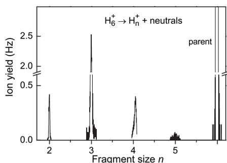
FIG. 5. Metastable dissociation of  $H_6^+$  into  $H_2^+$ ,  $H_3^+$ ,  $H_4^+$ , and  $H_5^+$  in the second field free region of the two-sector-field mass spectrometer (MIKE scan). Spontaneous (unimolecular) as well as collision-induced reactions contribute to the signal.
