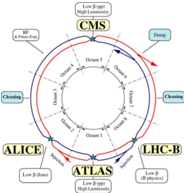
Figure 3. Schematic of the LHC. The red line represents the clockwise moving beam, and the blue represents the counterclockwise moving beam. The blue stars mark interaction points where the beams intersect and collisions occur, and also the locations of the four main detectors. Also marked is the site of the beam dump, where the beam can be safely diverted out of the collider ring into large blocks of graphite. Image courtesy of LHC Machine Outreach, <http://lhc-machine-outreach.web.cern.ch>.
