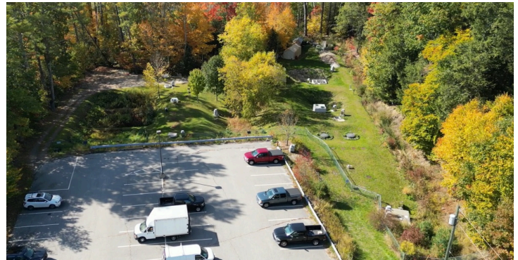
THE STORMWATER CENTER’S FIELD SITE, LOCATED AT THE EDGE OF A LARGE PARKING LOT ON UNH’S DURHAM CAMPUS, IS A STATE-OF-THE-ART TESTING FACILITY WHERE INNOVATIVE STORMWATER TECHNOLOGIES CAN BE EVALUATED IN A SIDE-BY-SIDE COMPARISON AS STORMWATER RUNS OFF THE ADJACENT LARGE PARKING LOT. PHOTO BY JOHN NADER.
