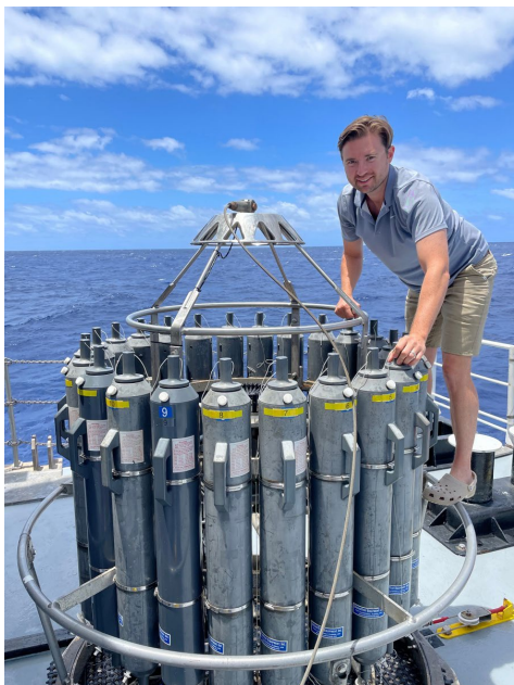
ROBERT LETSCHER COLLECTED SEAWATER USING THIS ROSETTE SAMPLER TO STUDY NUTRIENTS IN OCEAN DESERTS.
