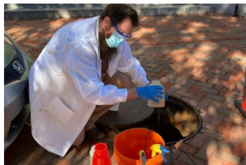
TECHNICIAN RETRIEVING SEWAGE SAMPLE FROM A MANHOLE ON UNH’S CAMPUS TO DETECT AND TRACK SARS-COV-2, THE VIRUS THAT CAUSES COVID-19. PHOTO CREDIT: PAULA MOUSER/UNH
