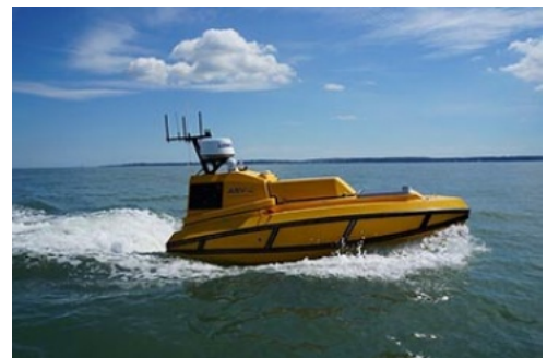
UNH’S AUTONOMOUS SURFACE VEHICLE KNOWN AS BEN (BATHYMETRIC EXPLORER AND NAVIGATOR), WILL HELP MAP THE OCEAN FLOOR TO HELP RESEARCHERS LOCATE AMELIA EARHART’S MISSING PLANE. PHOTO CREDIT: UNH
