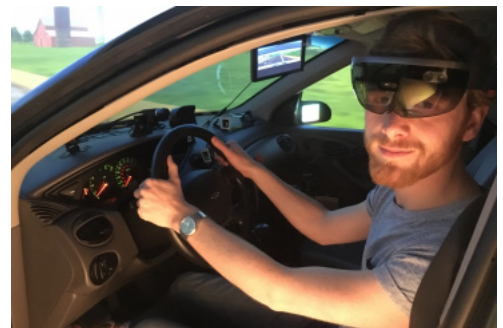
IN UNH’S DRIVING SIMULATOR, A RESEARCHER WEARS MICROSOFT HOLOLENS AUGMENTED REALITY GLASSES, WHICH OVERLAY VIRTUAL OBJECTS ON THE “WORLD” SHOWN BY THE SIMULATOR. COURTESY ANDREW KUN.
