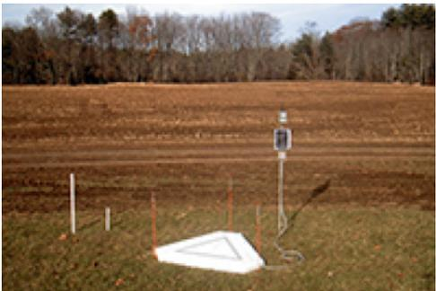
**A SNOWSCALE IS INSTALLED AT THE KINGMAN RESEARCH FARM IN MADBURY. THE SCALE, WHICH WILL MEASURE SNOWPACK, COMMUNICATES EVERY 30 MINUTES VIA WIRELESS MODEM TO COMPUTERS IN THE RESEARCHERS’ OFFICES WHERE THE DATA WILL BE COMPARED WITH INFORMATION COLLECTED FROM OTHER INSTRUMENTS AT THE FARM.**
