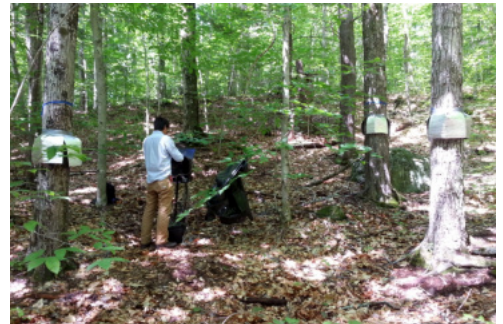
THESE TREES ARE INSTRUMENTED WITH SAP FLOW SENSORS THAT MEASURE HOW MUCH WATER THE TREES ARE USING DAY DURING THE GROWING SEASON. THE DATA ARE BEING DOWNLOADED TO A COMPUTER BY DOCTORAL STUDENT JOSE GUTIERREZ. CREDIT: HEIDI ASBJORNSEN/UNH
