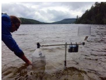
Doctoral student Amanda Murby monitors a lake aerosol collection system developed by UNH researchers on Lake Christine in Stark. Aerosolized cyanobacteria cells and toxins are collected on a fine glass fiber filter.
