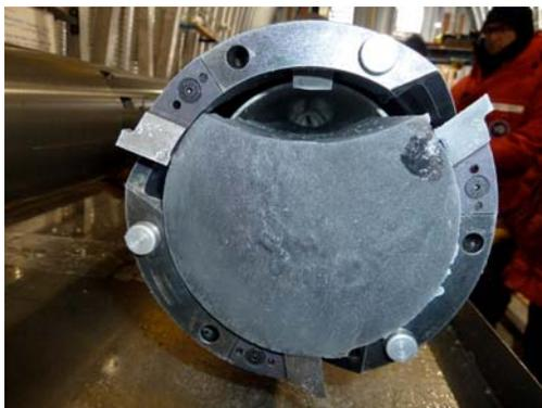
Caption: The first replicate core ever taken from the high side of an ice core borehole. The curvature on the top is the original borehole. The replicate core has a diameter of 4.25 inches. Photo by Jay Johnson, IDDO, University of Wisconsin-Madison.
