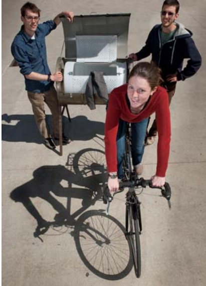
University of New Hampshire seniors Vincent Lyon, (from left), Britta Moore, and Garrett Cassidy – all mechanical engineering majors – fabricated a bicycled-powered washing machine that can clean a load of clothes in 30 minutes using only six gallons of water. Credit: Mike Ross, UNH Photographic Services
