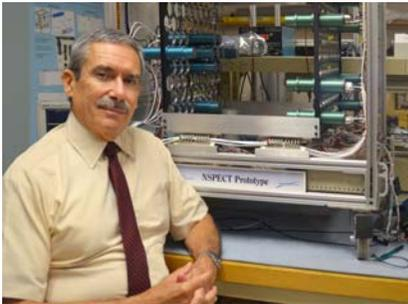
James Ryan beside the Portable Neutron Spectroscopy (NSPECT). The instrument was conceived, designed, and tested to image and measure sources of neutron radiation. Photo by Kristi Donahue, UNH-EOS
