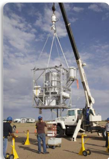
The GRAPE balloon payload shown during a power-up compatibility test on September 13 at the Columbia Scientific Balloon Facility in Ft. Sumner, NM. The larger vessel contains the GRAPE instrument. The smaller vessel on the right houses the FACTEL test instrument. Photo by Mark McConnell, UNH-EOS.
