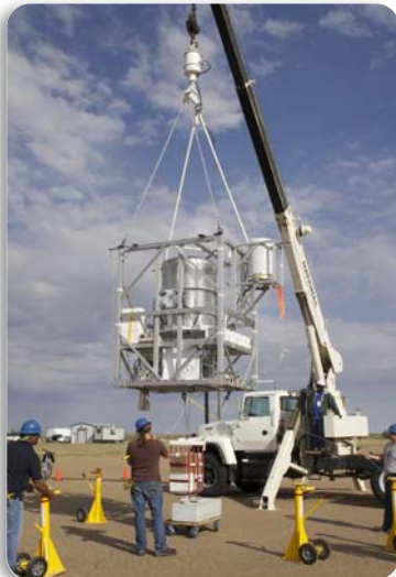
The GRAPE balloon payload shown during a power-up compatibility test on September 13 at the Columbia Scientific Balloon Facility in Ft. Sumner, NM. The larger vessel contains the GRAPE instrument. The smaller vessel on the right houses the FACTEL test instrument. Photo by Mark McConnell, UNH-EOS.
