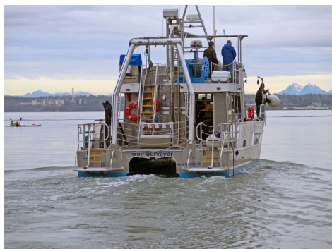
THE 48-FOOT ALUMINUM VESSEL WITH A CATAMARAN HULL HAS THE CAPABILITY TO DEPLOY SOPHISTICATED MULTI-BEAM ECHOSOUNDERS. ALL PHOTOS COURTESY OF CCOM/JHC.
