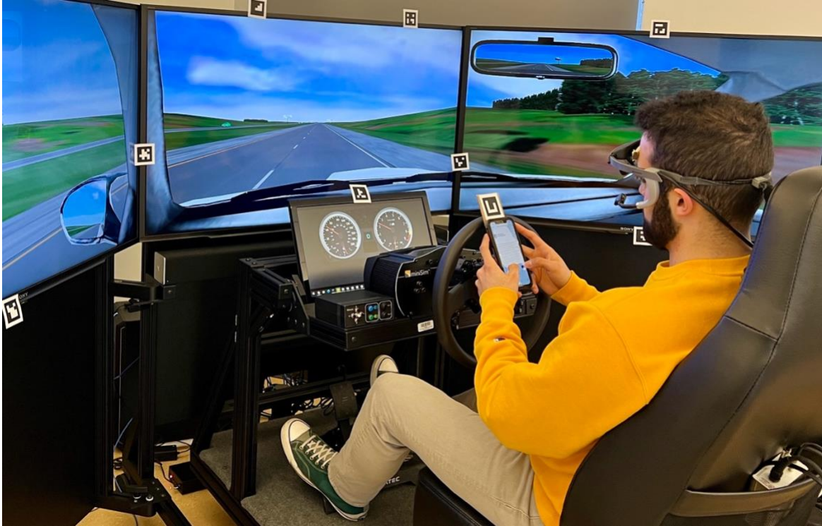
Figure 8 Experiment setup showing a participant wearing the eye tracker and using a smartphone to perform NDRT in the automated driving phase.
