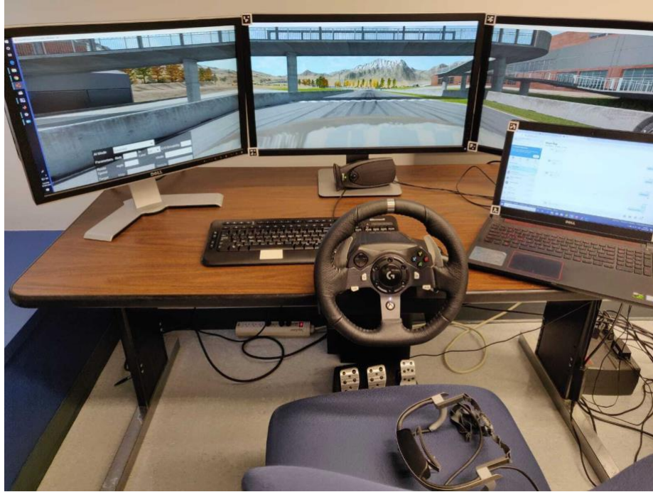
Figure 5 Experiment setup showing the driving simulator, the laptop used for performing the NDRT, and the eye tracker.
