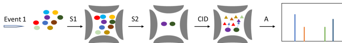
Scheme 3-2. S1: ions produced in electrospray ionization injected into ion trap, S2: isolation of desired ion in the ion trap, CID: collision-induced dissociation, A: mass analysis by scanning out of ions in the ion trap.
