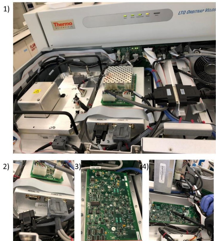
Figure 3-2 Overview of LTQ mass spectrometry after removing the cover, the left side was the vacuum manifold that enclosed ion optics, mass analyzer, and ion detection system. The PCB for mass analyzer rf voltage was next to the vacuum manifold. Photographs of measuring rf voltages 2) disconnected the electronic cables, 3) found the transformer components with code “TED” on the PCB, and 3) connected with the oscilloscope.
