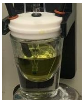
Figure 2.7. Faradaic EIS in ferri/ferrocyanide solution in UHP. The yellow color of the solution is due to the presence of in ferri/ferrocyanide ions.
