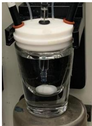
Figure 2.11. Non-Faradaic EIS in PBS buffer. The solution is clear because there are no ferri/ferrocyanide ions present.
