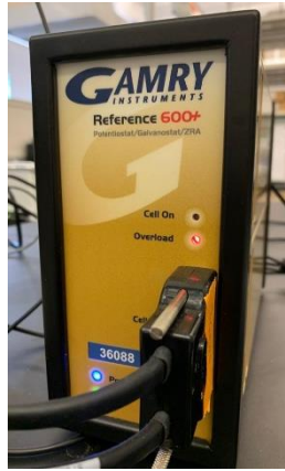
Figure 2.5. During a potentiostatic EIS experiment, the potentiostat (shown on the left) applies a sinusoidal potential and measures the current. (shown on the right)
