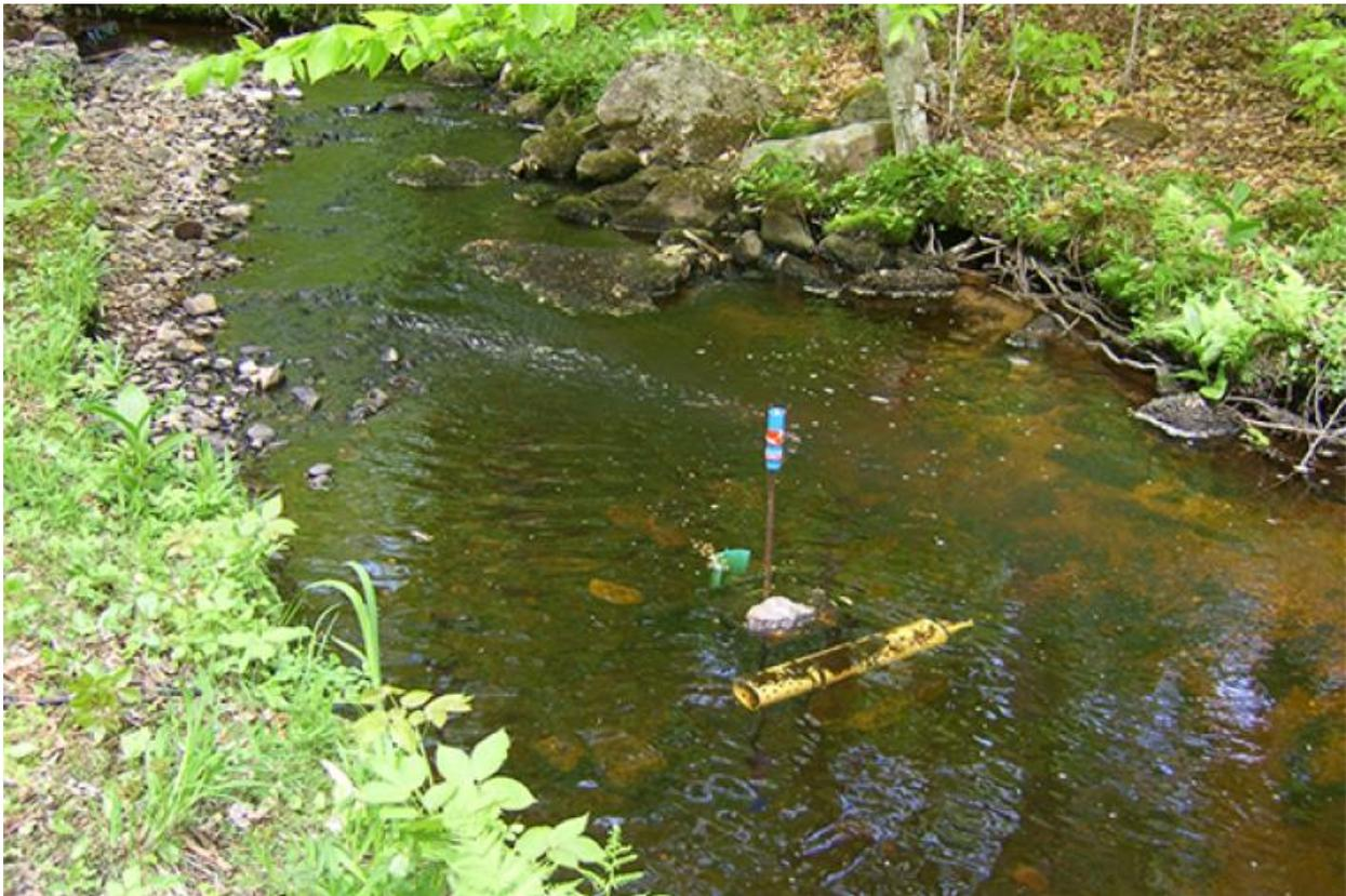
HIGH-FREQUENCY WATER QUALITY SENSOR TECHNOLOGY INSTALLED AT DOWST-CATE TOWN FOREST IN DEERFIELD, N.H. *PHOTO CREDIT: LISLE SNYDER*
