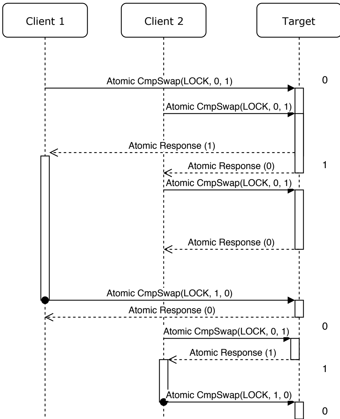
Figure 4-5: A lock mechanism using RDMA atomic operations.
