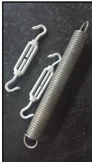
Figure 6.2: Spring and turnbuckles used for cross bracing photo credit: Kyle Wyatt 2015) .
