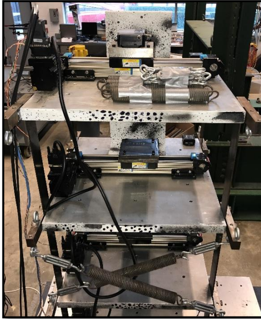
Figure 6.4: Test configuration for a damaged floor (6th) case.
