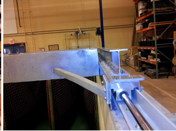
(b) Upgraded linear guides.
