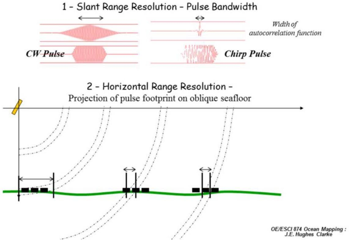
Figure 17: Range resolution model for a sidescan sonar system (Hughes Clarke, 2016). Higher slant range resolution is achieved with physically shorter pulses at a given frequency, or by utilizing chirp pulses which sweep through a band of frequencies, thus dramatically increasing range resolution by decreasing the width of the autocorrelation function. Horizontal range resolution is a function of grazing angle and increases with distance from nadir.
