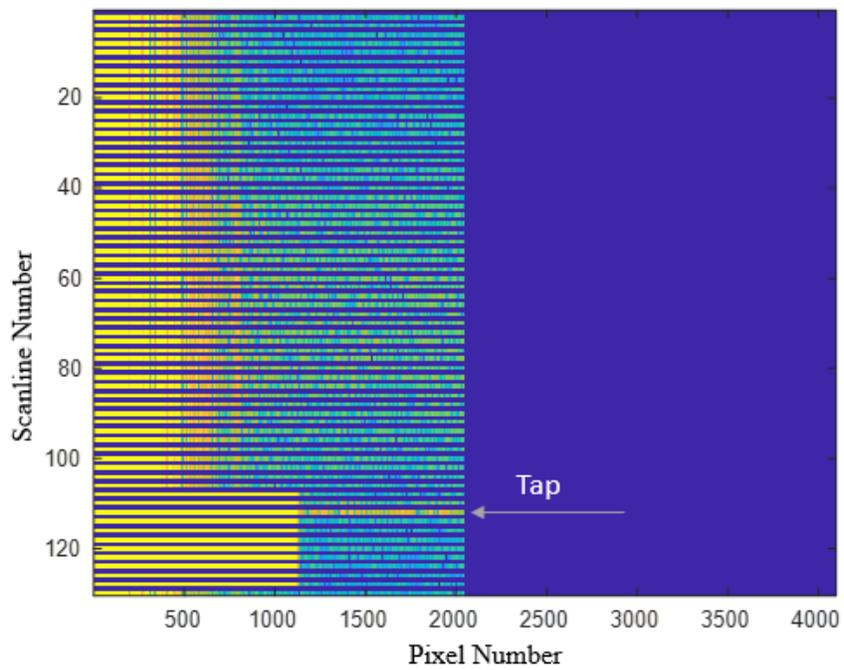
Figure 22: Transducer tap visualized in a reconstructed sidescan record using custom MATLAB code. Only the portside data is visualized because the starboard side of the transducer was face-down on the table, making the data irrelevant.
