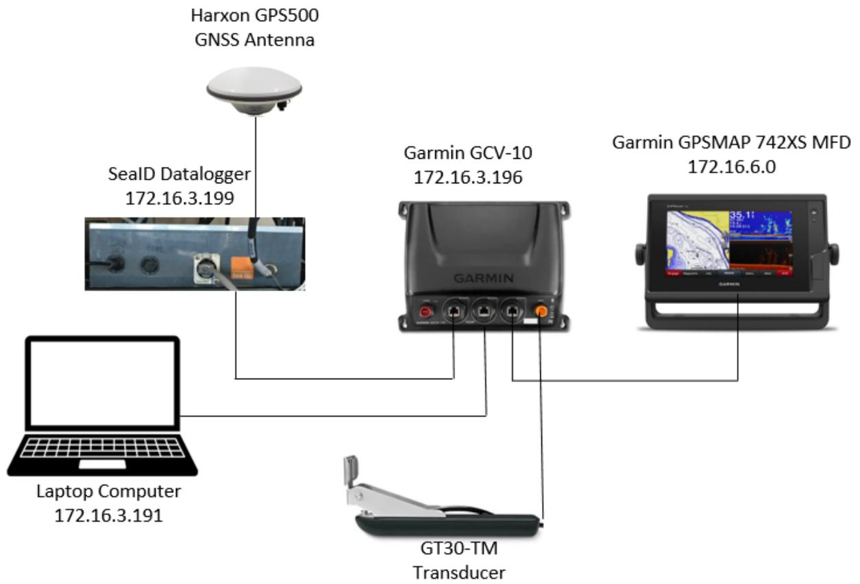
Figure 26: Hardware installation topology.
