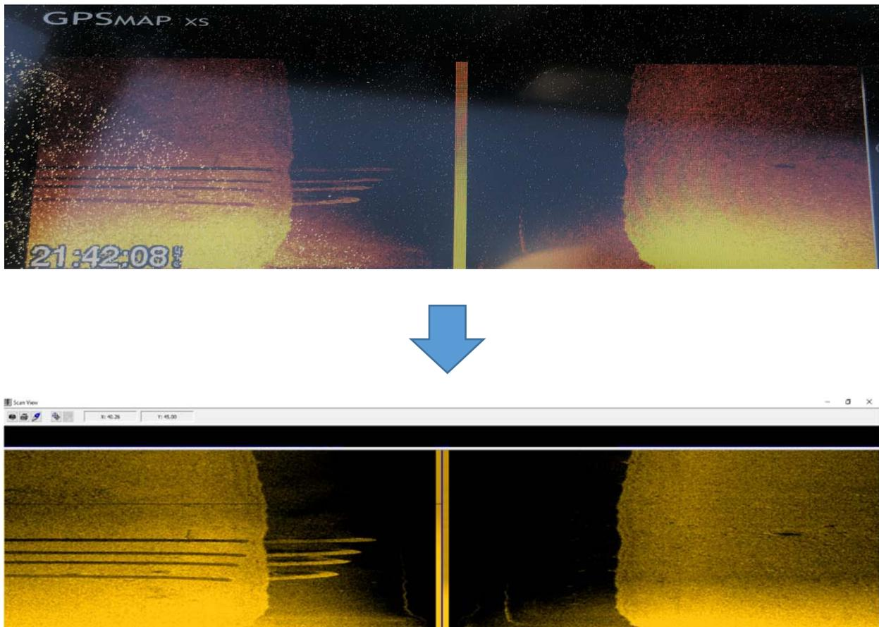
Figure 14: Photo of real-time sidescan imagery displayed on Garmin GPSMAP 742XS chart plotter (Top). Reconstructed Garmin GCV-10 sidescan imagery converted to XTF format using the XTF Converter code and rendered with the Hypack<sup>18</sup> Targeting and Mosaicking utility.
