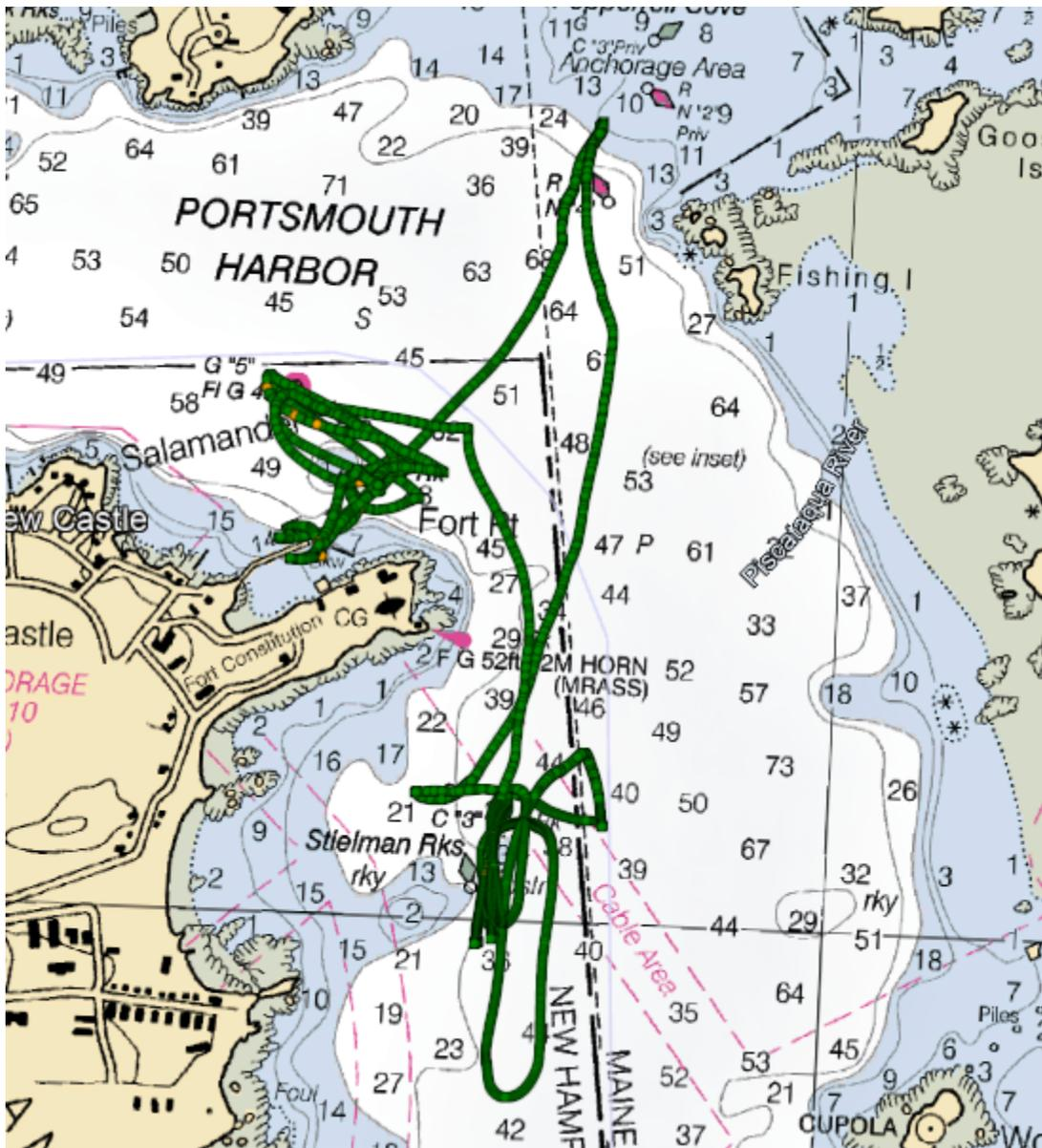
Figure 18: RVGS navigation record overlaid on NOAA Chart 13283 from data collection in the Piscataqua River to determine the Garmin GCV-10's optimized sidescan range setting in varying water depths.
