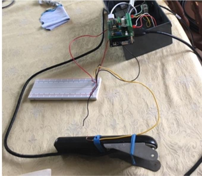
Figure 21: Pull-up resistor circuit implementation. The Odroid C2 computer with SeaID GNSS receiver was removed from the case to provide access to the Odroid's I/O pins.
