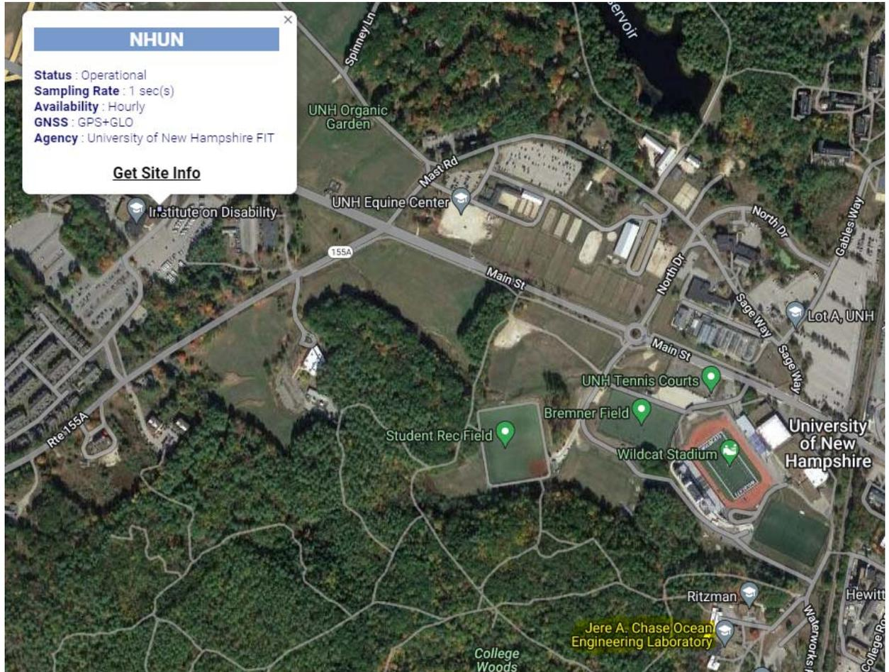
Figure 4: Satellite imagery showing relative locations of NOAA CORS Station (NHUN) and the Jere A. Chase Ocean Engineering Laboratory (highlighted in yellow), where the experiment took place. The baseline distance between the two antenna locations is 1277m. Image taken from NOAA CORS Map online: [https://geodesy.noaa.gov/CORS\\_Map/](https://geodesy.noaa.gov/CORS_Map/).
