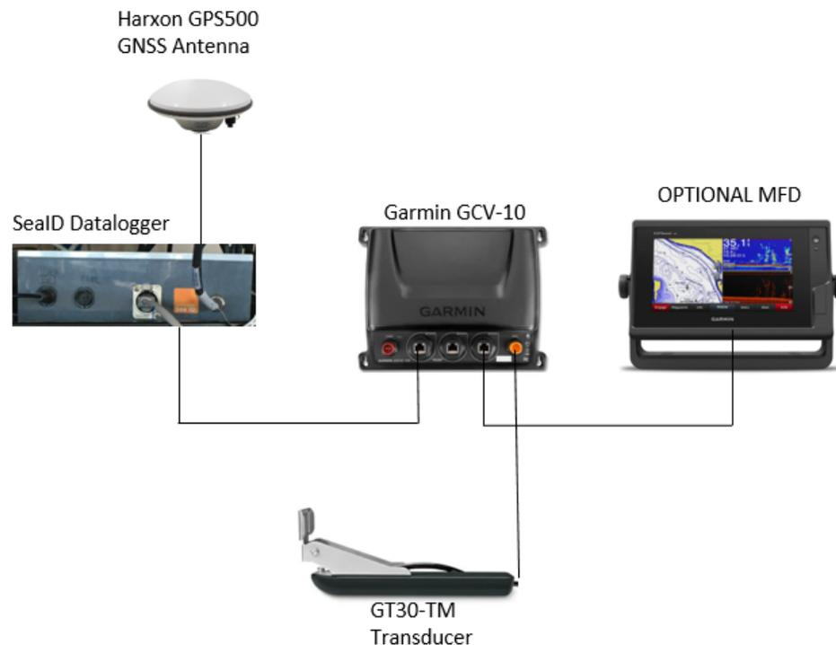
Figure 15: Physical installation schematic for logging sidescan data using the SeaID prototype TCB datalogger. The Garmin MFD is optional because the echosounder can be controlled solely with the TCB Datalogger if there is no need for a real-time data display.
