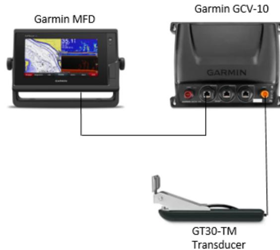
Figure 8: Generic Garmin GCV-10 installation schematic.
