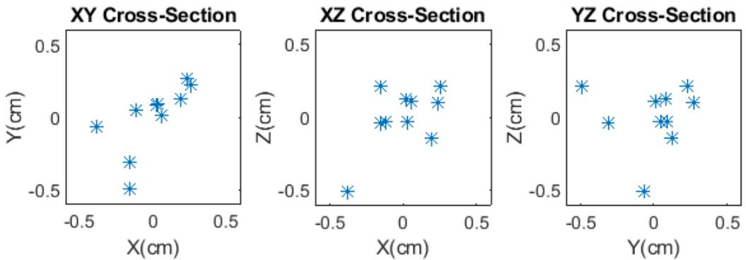
Figure 7: : Two-dimensional cross sections of 10 single point ( $\approx 24$ hr) position solutions from the Harxon GPS500 antenna and SeaID receiver presented in East-North-Up (ENU) Cartesian coordinate system, whereas the East-North (XY) plane is the local horizon plane, and the origin is the average estimated location of the antenna for the entire set of observations. The mean was removed from each axis for simplicity of interpretation.
