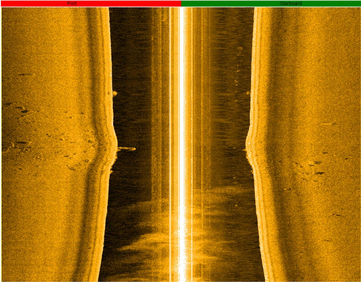
Figure 40: Waterfall view of Garmin GCV-10 sidescan record (Figure 39) with water column collected at ~4kts, 20m scan range, 800kHz, in vicinity of Stielman Rocks, Portsmouth Harbor, New Hampshire.
