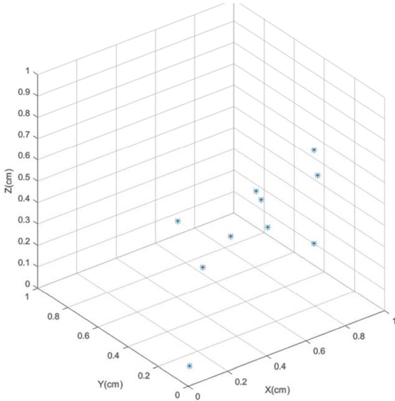
Figure 6: Single point (24hr) position solutions from the Harxon GPS500 antenna and SeaID receiver displayed in Earth Centered Earth Fixed (ECEF) Cartesian coordinate system with the mean position removed from each axis for simplicity of interpretation.
