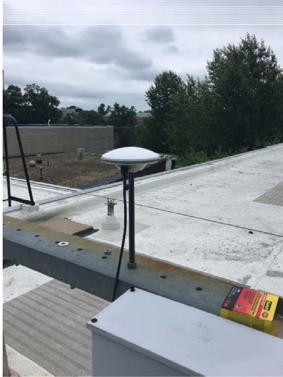
Figure 3: Harxon GPS500 antenna mounted on the rooftop of the CCOM wing of the Chase Ocean Engineering building.
