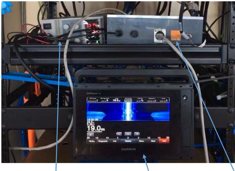
Figure 29: 12VDC Power Supply, Garmin 742XS multifunction display and TCB Datalogger installed on RVGS.
