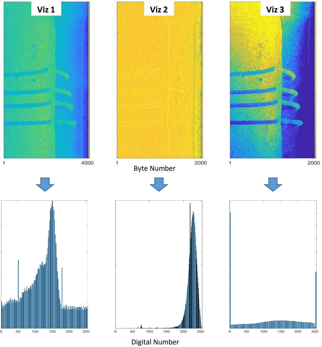
Figure 12: Three visualizations of the same portside sidescan record of four bridge pilings produced by the Garmin GCV-10 (Top) and their corresponding histogram (Bottom).
