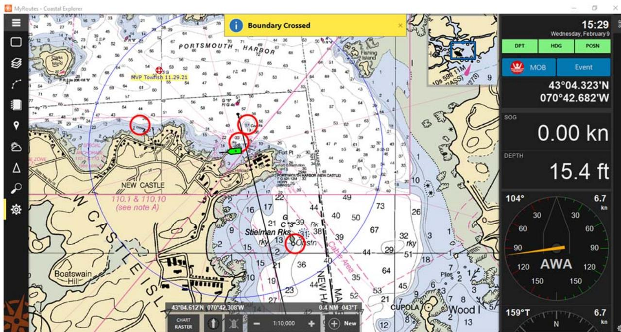
Figure 36: Four boundary circles (red) displayed on *R/V Gulf Surveyor*'s chart plotter running Rose Point Coastal Explorer software, marking demonstration targets of interest.
