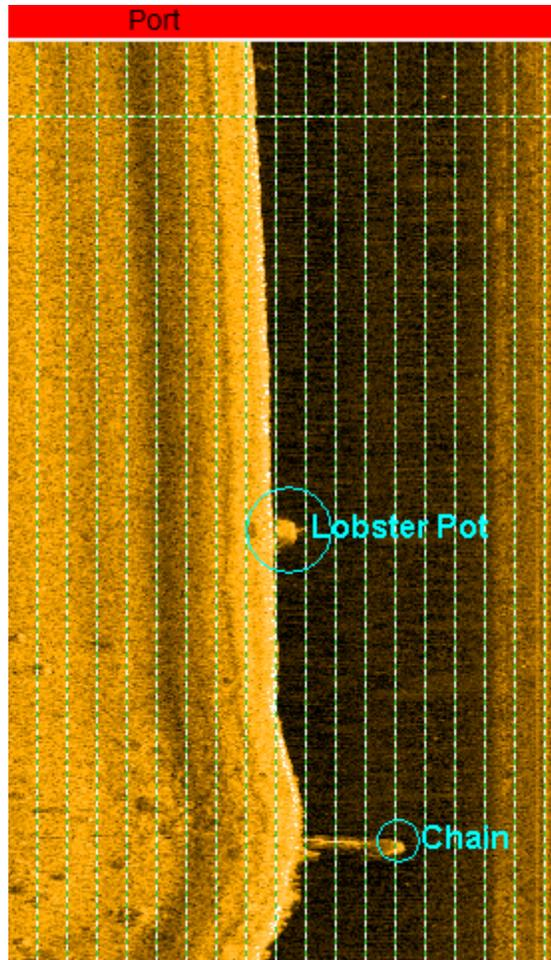
Figure 41: Zoomed in view on two targets visible in Figure 40, with horizontal scale lines at 1 meter interval starting from nadir. Notice the system's ability to image the buoy line coming off the lobster pot, and the mooring chain for USCG navigation buoy GC'3'.
