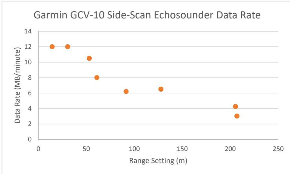
Figure 45: Range is the distance from nadir to one edge of the side-scan swath. Effectively half the total swath width. It's likely that changes in ping rate account for changes in data volume but proving that relationship was outside the scope of this project.
