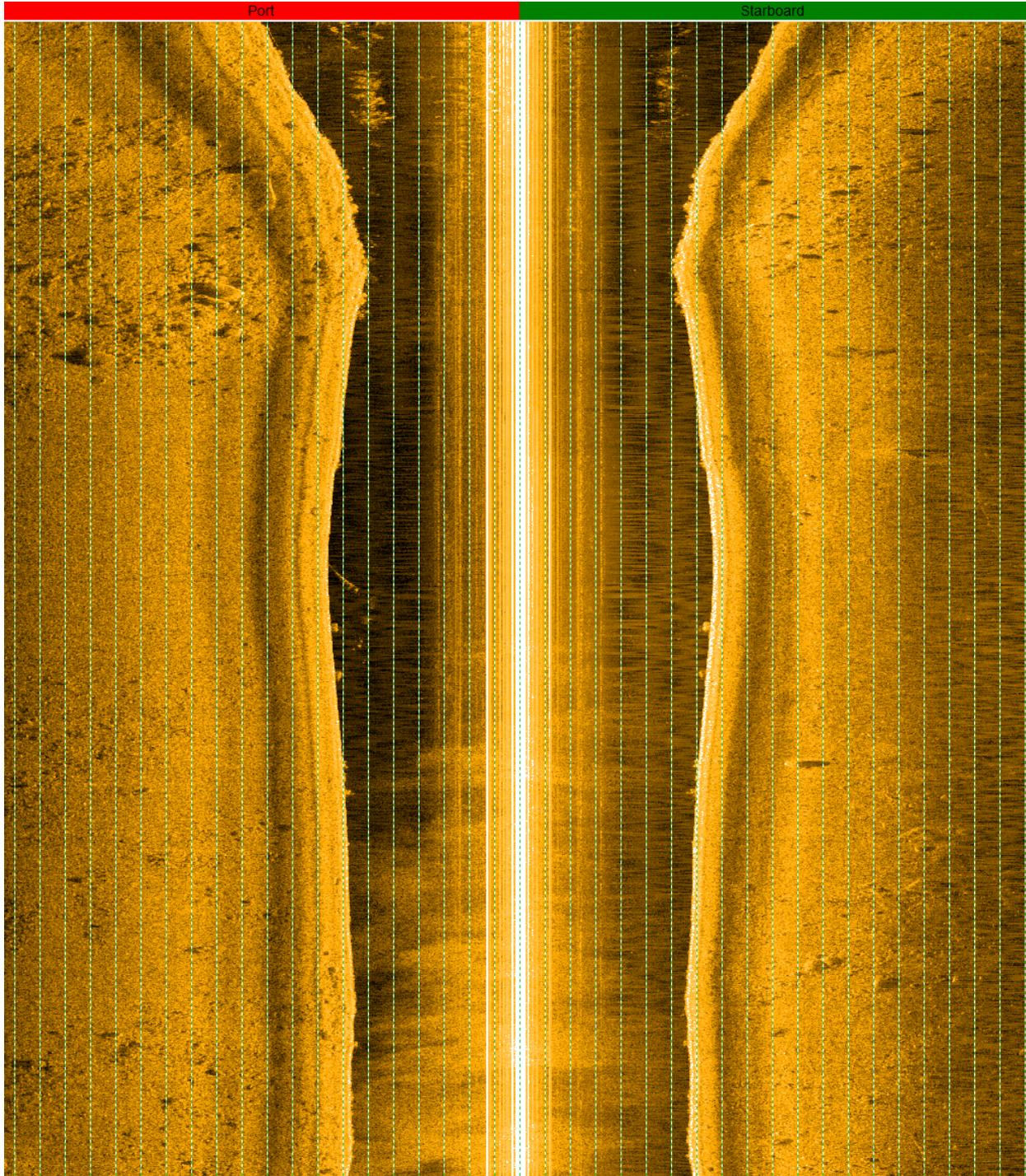
Figure 43: Waterfall view of sidescan record from Figure 42. Horizontal scale lines overlaid at 1m interval for scale.
