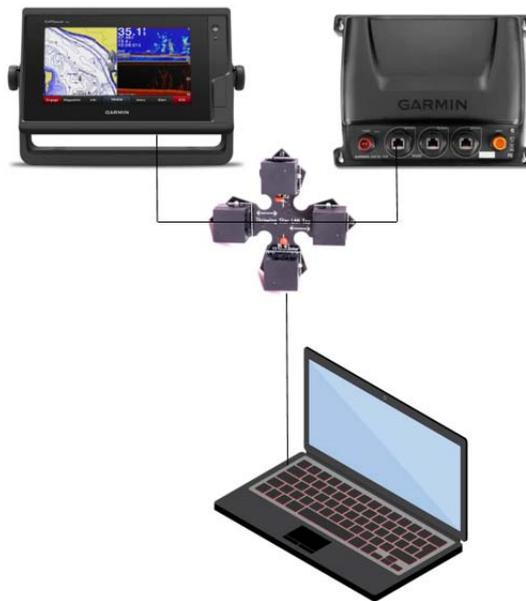
Figure 9: Wiring schematic for passively sniffing network traffic between the echosounder processor and chart plotter using a Throwing Star LAN Tap and a laptop running Wireshark.
