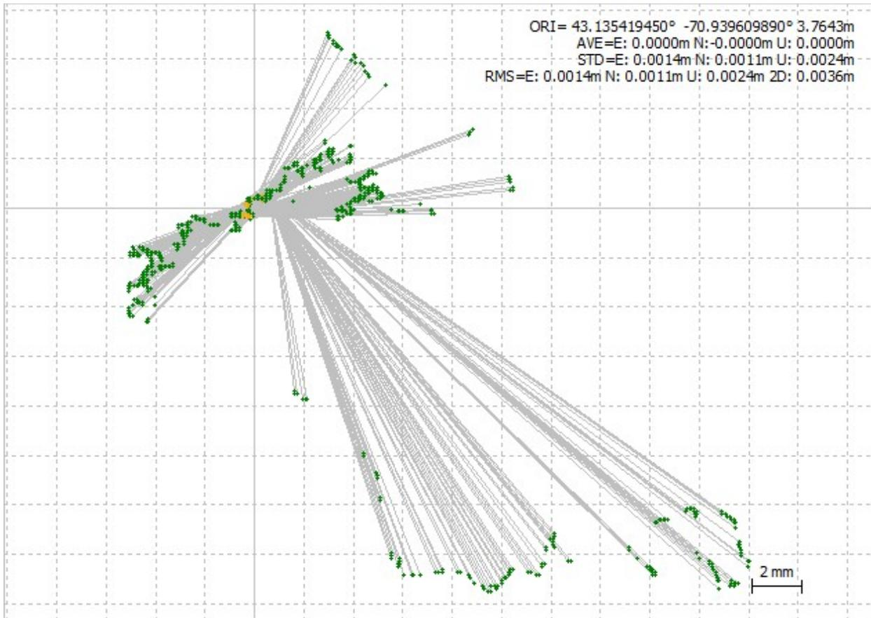
Figure 5: Geographic distribution of post-processed positioning solutions using RTKLIB from 2018-08-09 00:00:00 GPST through 2018-08-09 23:59:59 GPST. Green are fixed ambiguity solutions, yellow are floating point solutions.
