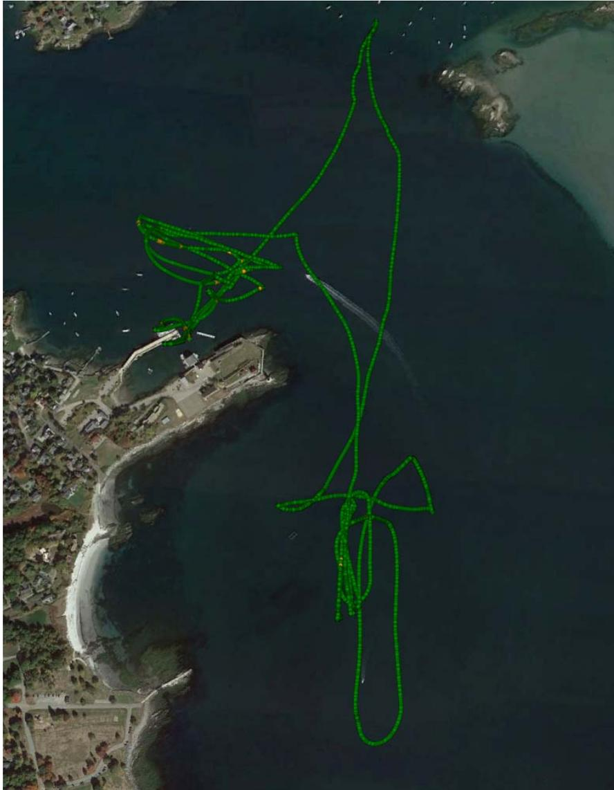
Figure 37: Post processed 3D position solutions from autonomous data collection generated by RTKLIB and visualized in Google Earth. Green dots indicate RTK fix- and yellow dots indicate RTK float-solutions.
