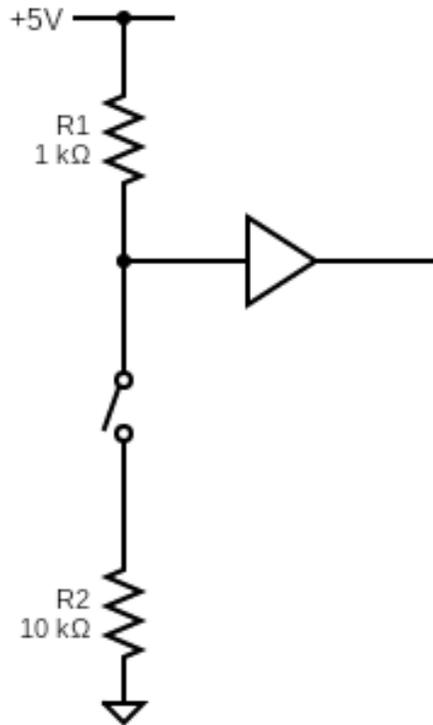
Figure 20: Pull-up resistor circuit diagram. The TCB datalogger utilizes an Odroid C2 computer capable of 5VDC output on Pin 1. Header pin #16 (GPIO #236) registers LOW when the circuit is completed at the transducer.
