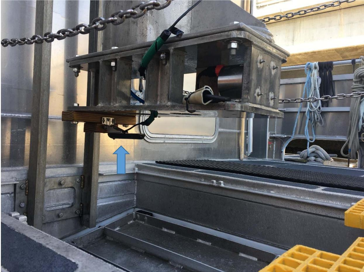
Figure 28: Garmin GT30-TM transducer installed on R/V *Gulf Surveyor's* primary transducer strut. The strut is aligned with the vessel's centerline and can be vertically articulated from the stowed position (shown), to a deployed position which secures the transducer submerged below the hull, clear of bubble wash.
