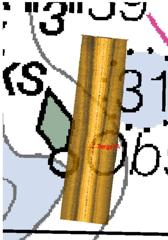
Figure 31: Georeferenced sidescan record with water column removed from latency test site A, overlaid on NOAA chart 13285 (top). Sidescan waterfall display from latency test site A, notated with gridlines at 1m interval for scale (bottom). The target position used for the test is notated in both images.
