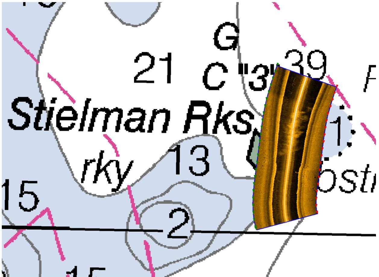
Figure 39: Garmin GCV-10 sidescan record with water column collected at ~4kts, 20m scan range, 800kHz, in vicinity of Stielman Rocks, Portsmouth Harbor, New Hampshire. Overlaid on NOAA chart 13283.
