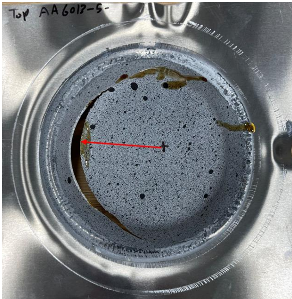
Figure 1.18: Failed specimen from a cup drawing test with shim placed at +X.
