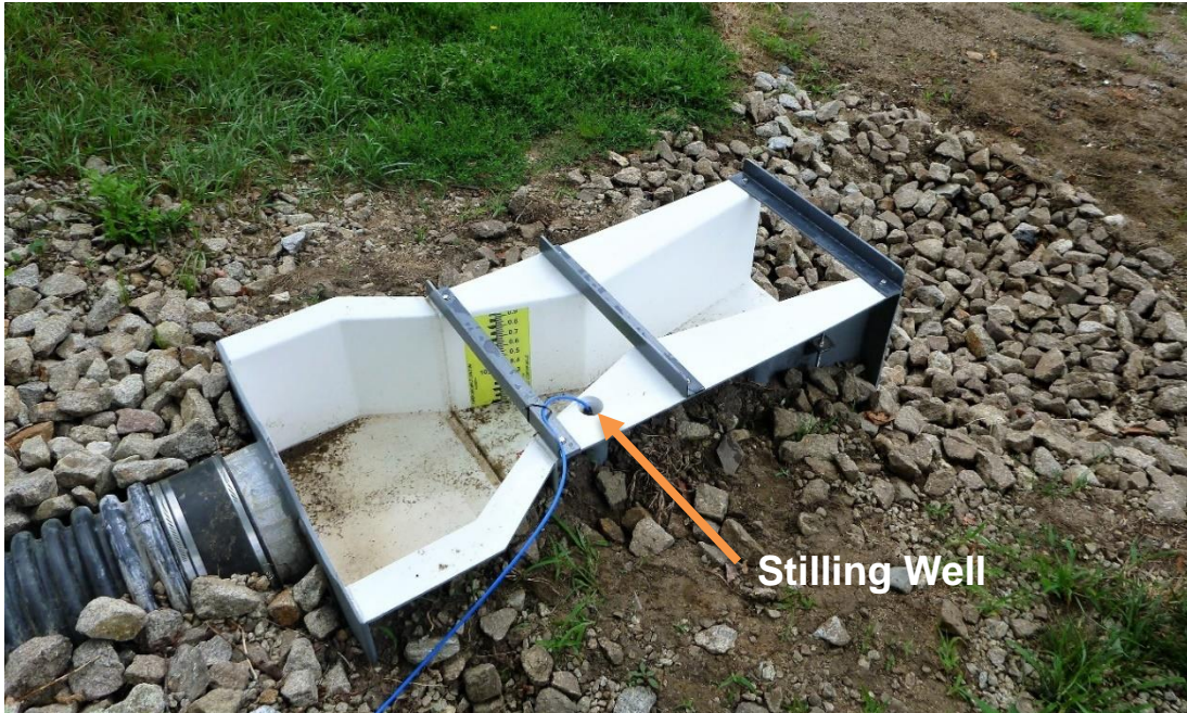
Figure 14: Inlet monitoring using an OCF 36x8 inch Cutthroat Flume. The blue line seen at the bottom center of the image is the data line for the pressure transducer located in the stilling well.
