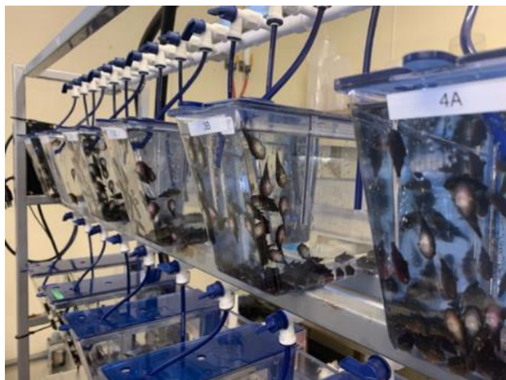
Figure 3.1. The experimental flow-through seawater system used in both trials.
