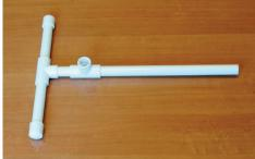
**Step 6:** Attach the PVC coupling to the other end of the pipe piece.
