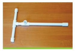
**Step 7:** Insert a 12" pipe piece into the open connection of the PVC tee connector. This will be the launch tube.
