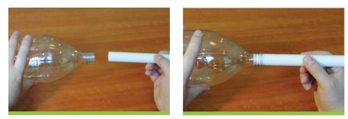
**Step 9:** Secure the pipe to the bottle using a 4" long piece of duct tape.
