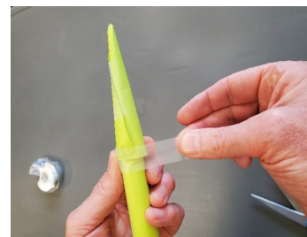
Figures 18-19. Tape nosecone to tip with tape
