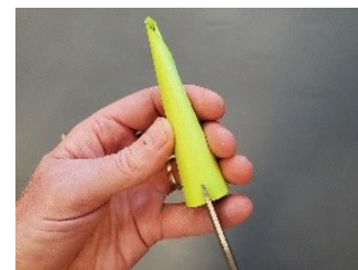
Figures 14-17. Curl to form nosecone and tape seam
