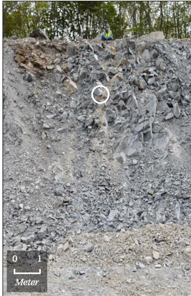
Figure 5.2. The preliminary test site in a recently blasted rock cut in Dover, NH. The white circle shows the test block position in the captured video frame.
