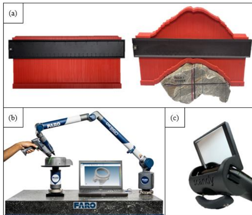
Figure 3.2. (a) Plastic contour gauge, (b) Faro 3D ScanArm ( https://www.faro.com ), and (c) Scandy Pro Lookout ( https://www.scandy.co/apps/scandy-pro ).
