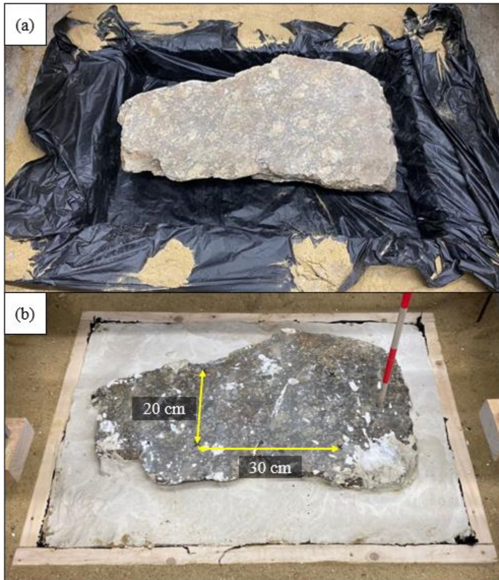
Figure 3.14. (a) Preparation of the test pit for the drop tests on rock, and (b) experimental setup.
