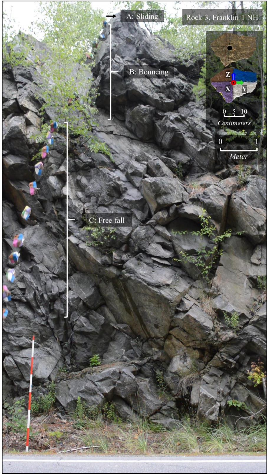
Figure B.35. Rockfall trajectory: rock 3, Franklin 1 NH.
