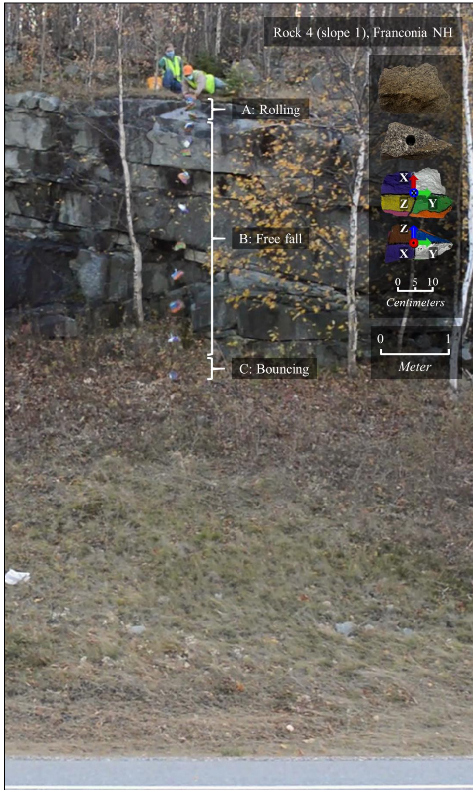
Figure B.20. Rockfall trajectory: rock 4 (slope 1), Franconia NH.
