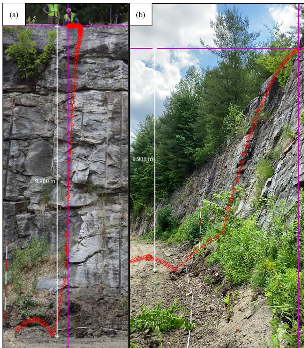
Figure 4.4. Frontal and lateral trajectories were determined using Tracker software (reference rock, Keene NH).
