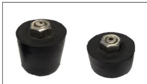
Figure 3.9. Expandable rubber plugs and through-hole screws: original length (left) and shortened (right).
