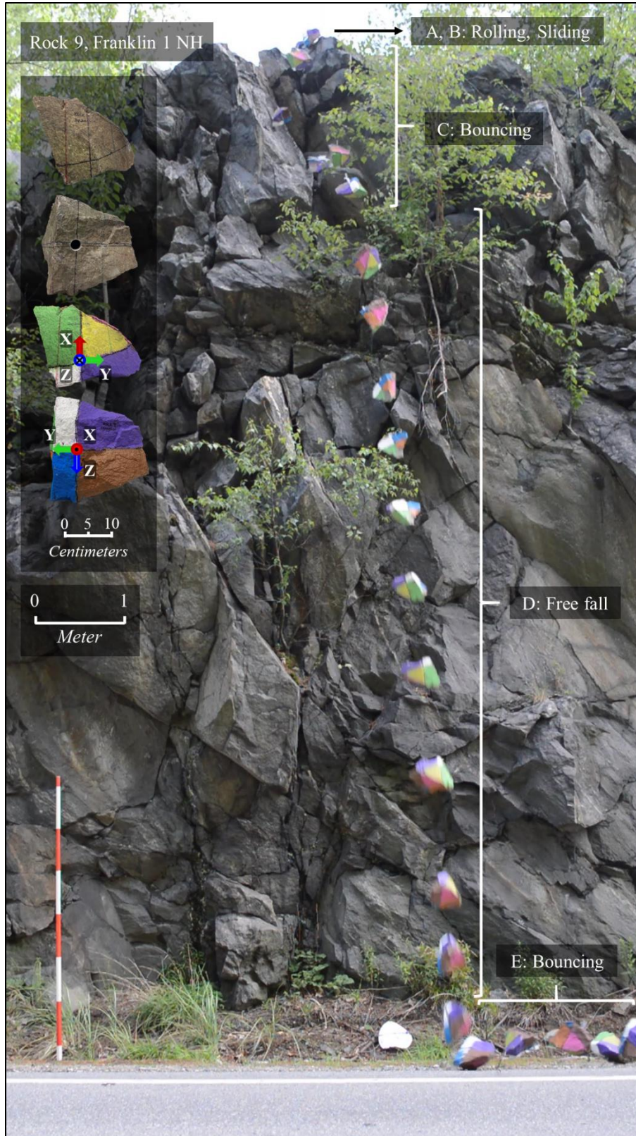
Figure B.40. Rockfall trajectory: rock 9, Franklin 1 NH.
