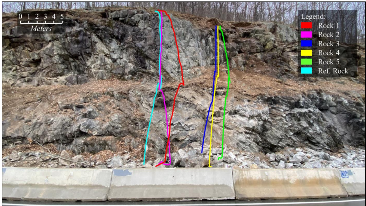
Figure 5.62. Rockfall trajectories: Townshend VT. Please note some horizontal distortion in the trajectories due to the camera position and wide lenses to capture the entire slope. The detailed trajectories show accurate positions.
