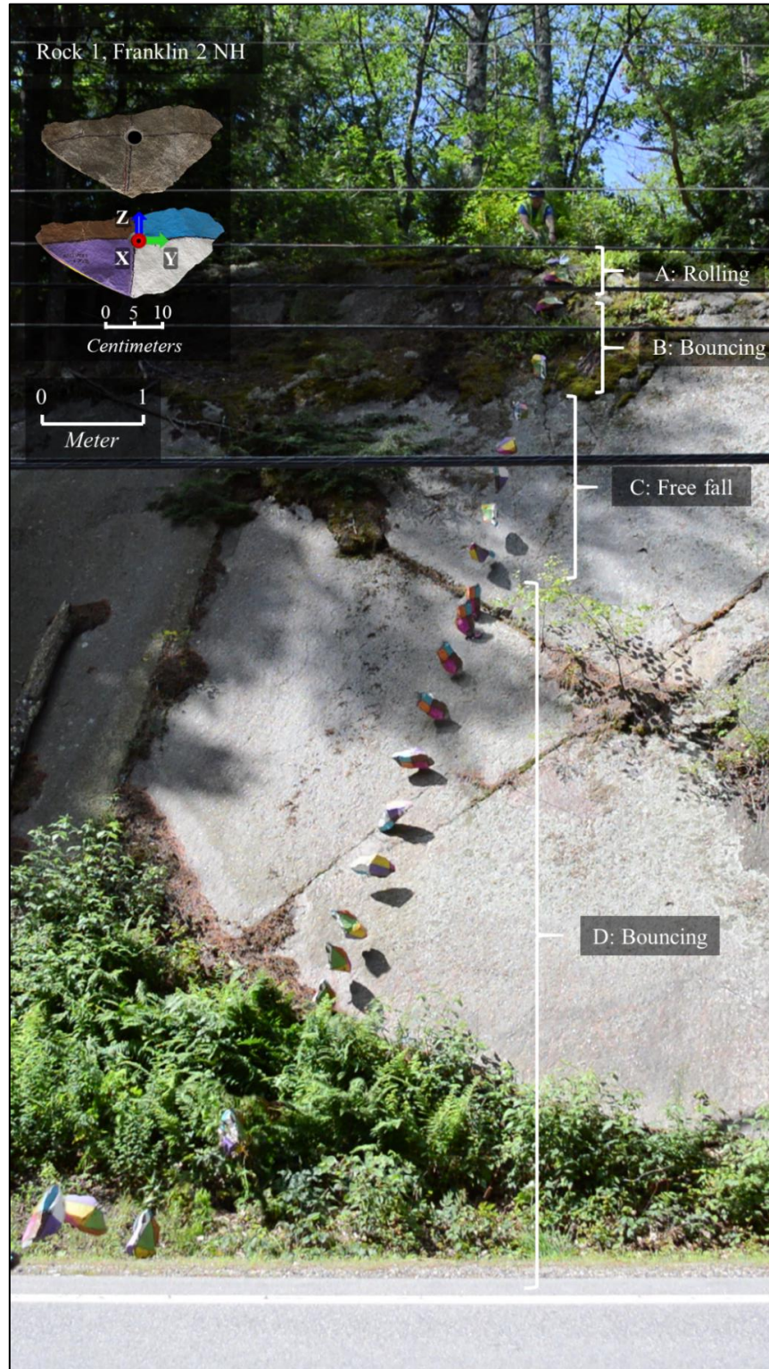
Figure B.42. Rockfall trajectory: rock 1, Franklin 2 NH.
