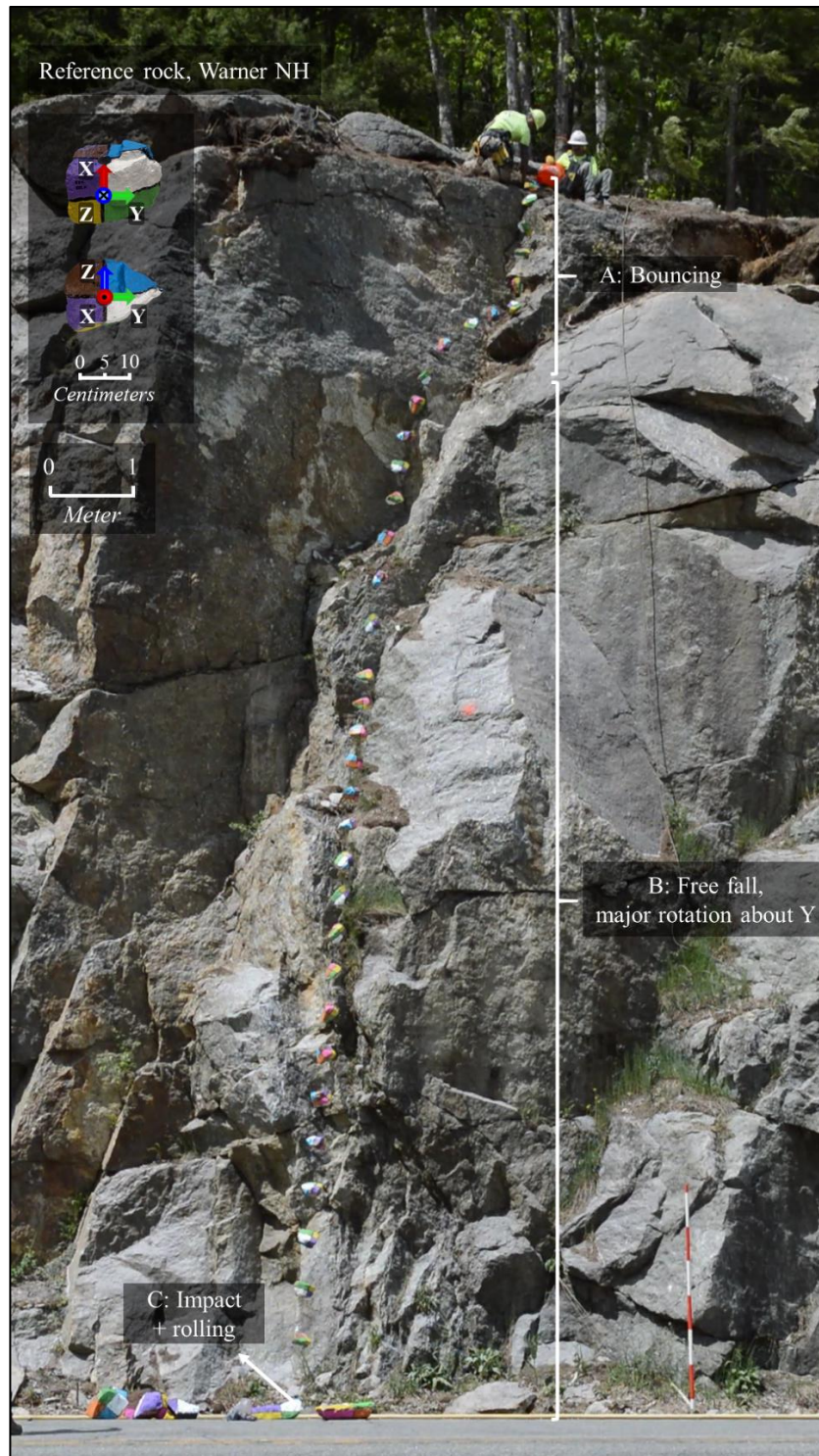
Figure 5.81. Rockfall trajectory: reference rock, Warner NH.
