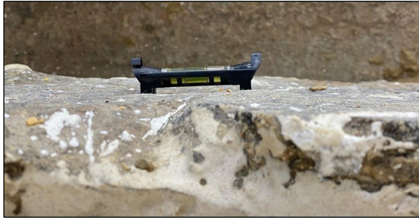
Figure 7.9. Small inclination of the natural rock at the point of contact (below the spirit level).
