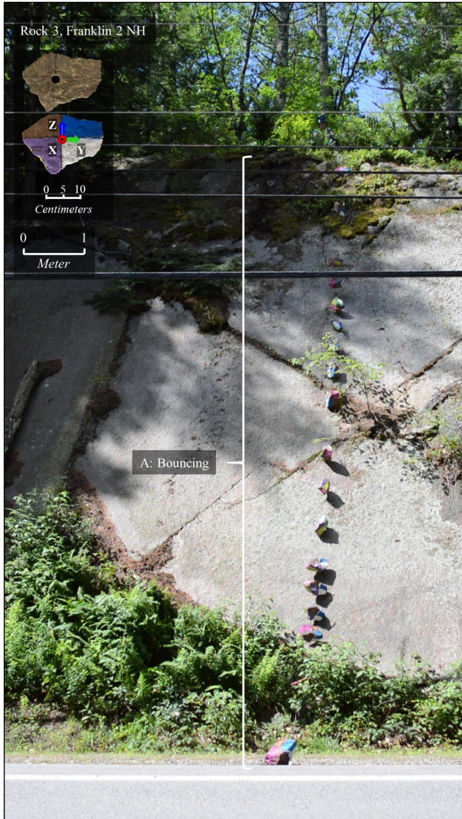
Figure B.45. Rockfall trajectory: rock 3, Franklin 2 NH.
