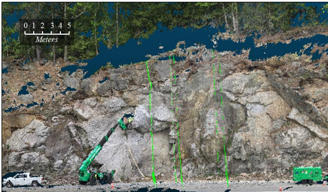
Figure 8.8. Three-dimensional digital model for the rock cut in Warner, NH.
