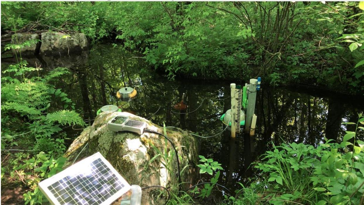
*Cart Creek, pictured above, is one of the headwater sites, including in situ sensors and water table gauge (right), the YSI instrument that measures stream parameters such as temperature, dissolved oxygen, pH, and conductivity (on the rock) and floating chambers (left) which help to capture and estimate greenhouse gas flux.*
