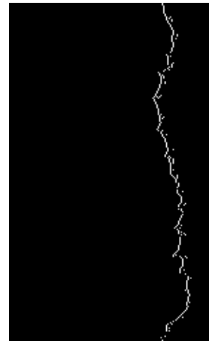
Figure 2.49: Identified Edges of LP-S3, Threshold = 12
