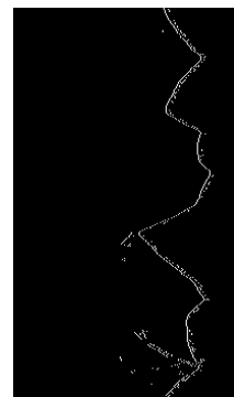
Figure 3.64: 200 x 350 LPS Edges, Failed Path
