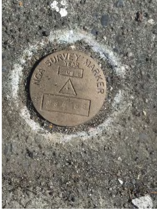
Figure 9a. Post-cruise gravity tie monument at the University of Washington Marine Sciences Bldg. dock, Seattle.
