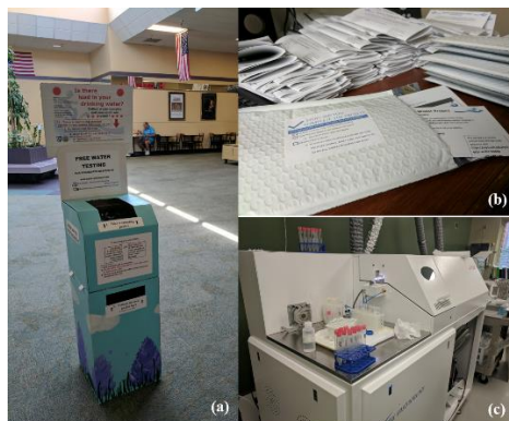
Figure 2. (a) Two-level, cardboard informational kiosks were designed to attract the attention of passersby and provide key information to participate in the project. (b) Sampling packets were housed in pre-paid mailing envelopes to allow for easy return upon completion. (c) Returned samples were analyzed for lead concentration using an inductively coupled plasma mass spectrometer at a University of New Hampshire lab.
