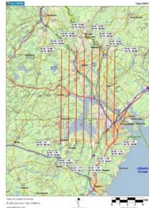
Eight lines oriented approximately north-south with a 30% overlap were collected in each survey with a ground resolution of 2.5 m.
