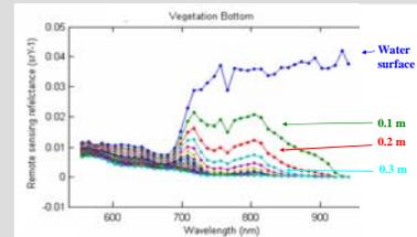
In natural environments the spectral signature from the seafloor is often complicated due to the water-column attenuation. Both the water column and bottom contribute to the water-leaving radiance with their relative contributions being modulated by water depth. The attenuation changes as a function of wavelength.
