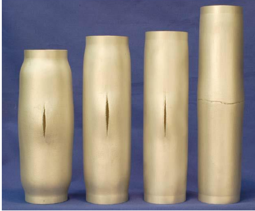
Figure 1.9: Burst failure in Al-6062-T6 obtained in free expansion experiments with different ratios of pressure and axial force, tested by Korkolis, Kyriakides [18].
