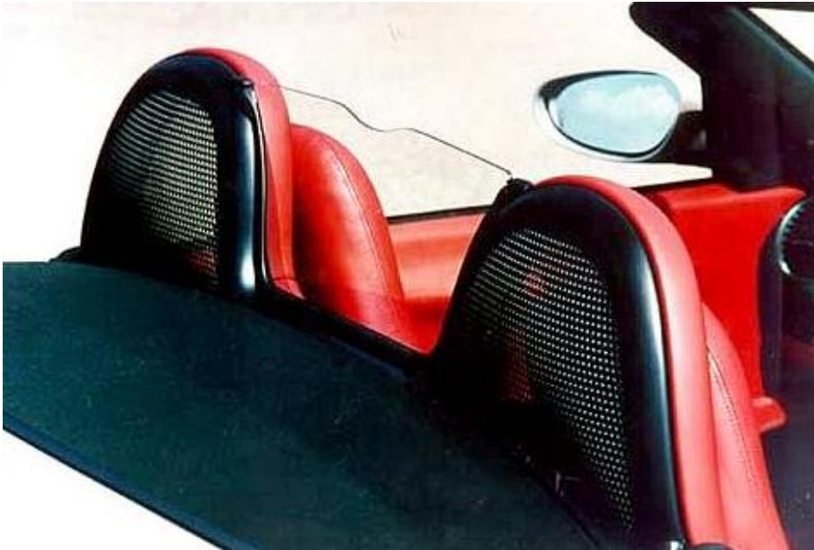
Figure 1.4: An example of how hydroformed components are being used in the transportation industry. This particular 2-piece roll bar is from a convertible Porsche Boxster ( http://www.schulergroup.com/ , http://www.autospeed.com/ ).
