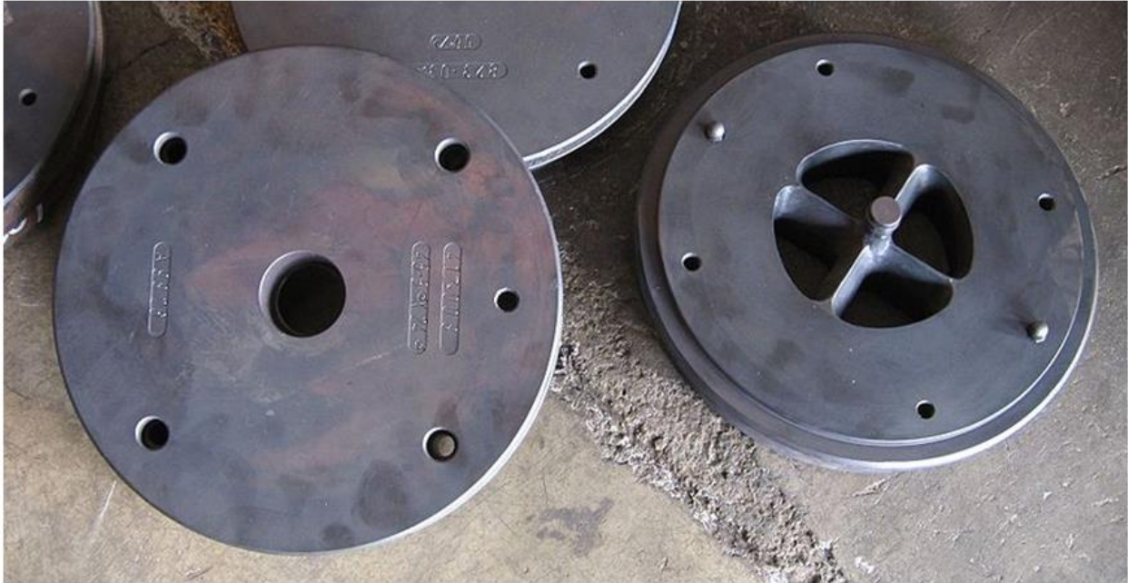
Figure 3.2: Example of the extrusion dies for making tubes (not actual die used for the Al-6061-T4 of this work). Legs holding the billet cause cold-welds in the extrusion profile [27].
