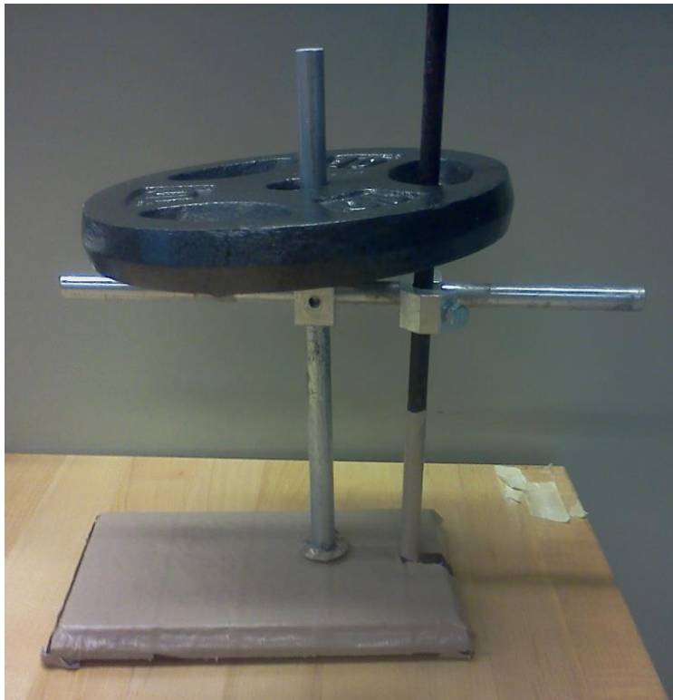
Figure 69: The device used to apply weight to a small area
