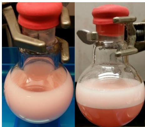
Figure 14: Phase transfer ligand exchange reaction between OA-CdSe (in toluene) and L-Cys (in water). During the reaction (left) the mixture forms an emulsion. After letting the mixture stand (right), the aqueous phase settles out, containing the newly-formed L-Cys-CdSe as clearly indicated by the color.
