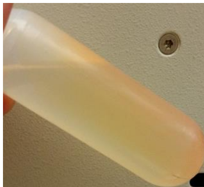
Figure 15: L-Cys-CdSe precipitated on the side of the centrifuge tube
