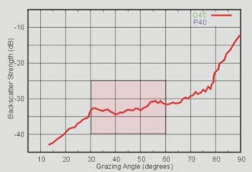
Fig. 4. Typical backscatter versus grazing angle curve for the EM 1000 data collected on the Eel River Margin. Only the sector between 30 and 60 degrees was used for these analyses.
