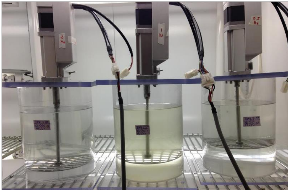
Figure 2 | Image of oscillating grid tanks in the light and temperature controlled incubator. Grids were set to oscillate at a specific frequency to generate homogenous turbulence in the tanks.
