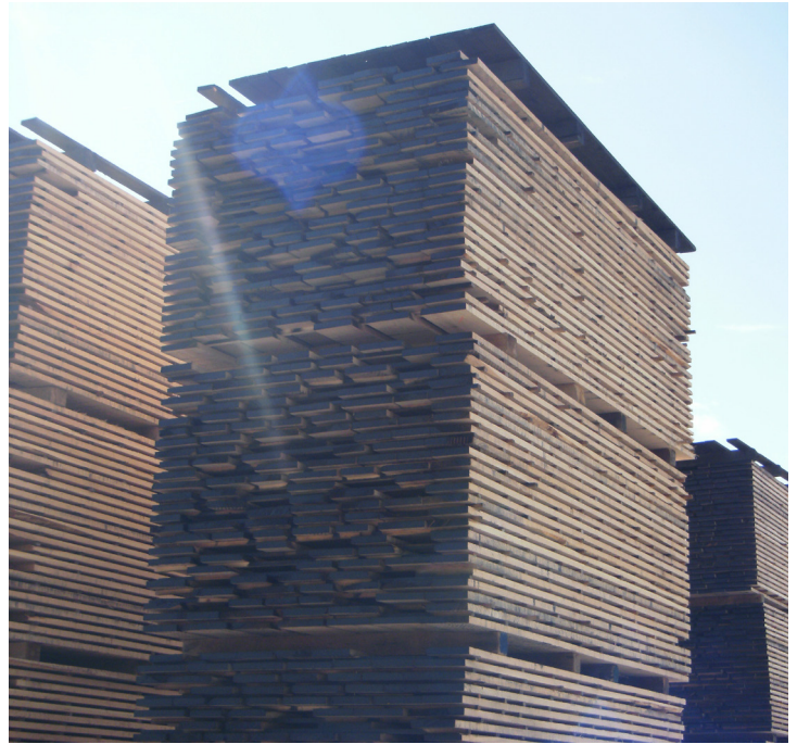
Figure 4. The boards missing from the pile covers in the above photograph can easily be replaced with low-grade lumber that is generated at the sawmill. Photo source: Patrick M. Rappold.
