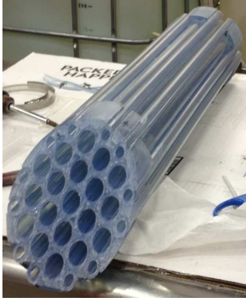
Figure 3.3 Pipe array static inline mixer before placement in pipe showing blocked surface area
