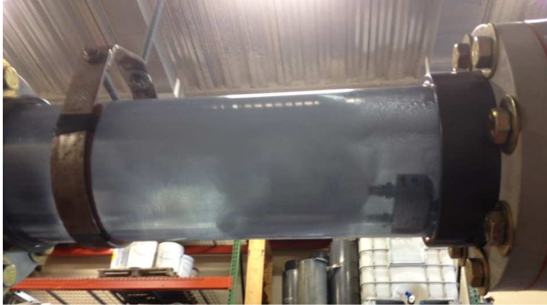
Figure 3.2 Reactor design with no static mixers, double nozzle placed on bottom of reactor for optimal air coverage
