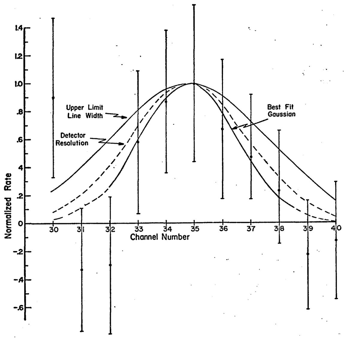
Figure IV-15. The flare peak at 0.51 MeV and the best fit Gaussian curve with a FWHM of 7.4%. Also shown are peaks with widths corresponding to the detector resolution and to the (2 $\sigma$ ) upper limit linewidth.
