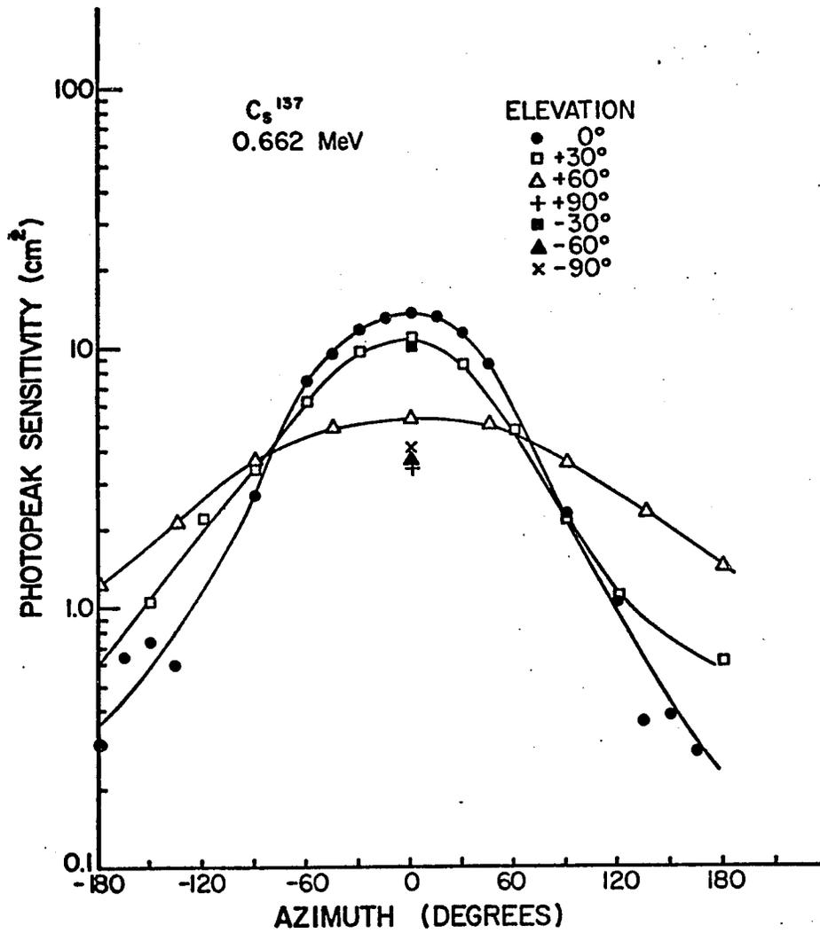
Figure II-3. Variation of detector sensitivity (cm<sup>2</sup>) with azimuth and elevation for a 0.662 MeV ( $Cs^{137}$ ) point source.
