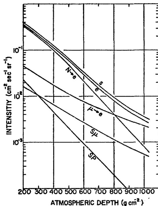
Figure A-1. Vertical intensities versus atmospheric depth of the soft component (S) and its subcomponents;  $S = e + \pi\mu + sp$ ,  $e$  (electrons) =  $N \rightarrow e$  (electrons from  $\pi^0$ ) +  $\mu \rightarrow e$  (electrons from the knock-on and decay processes of muons), (Hayakawa, 1969).
