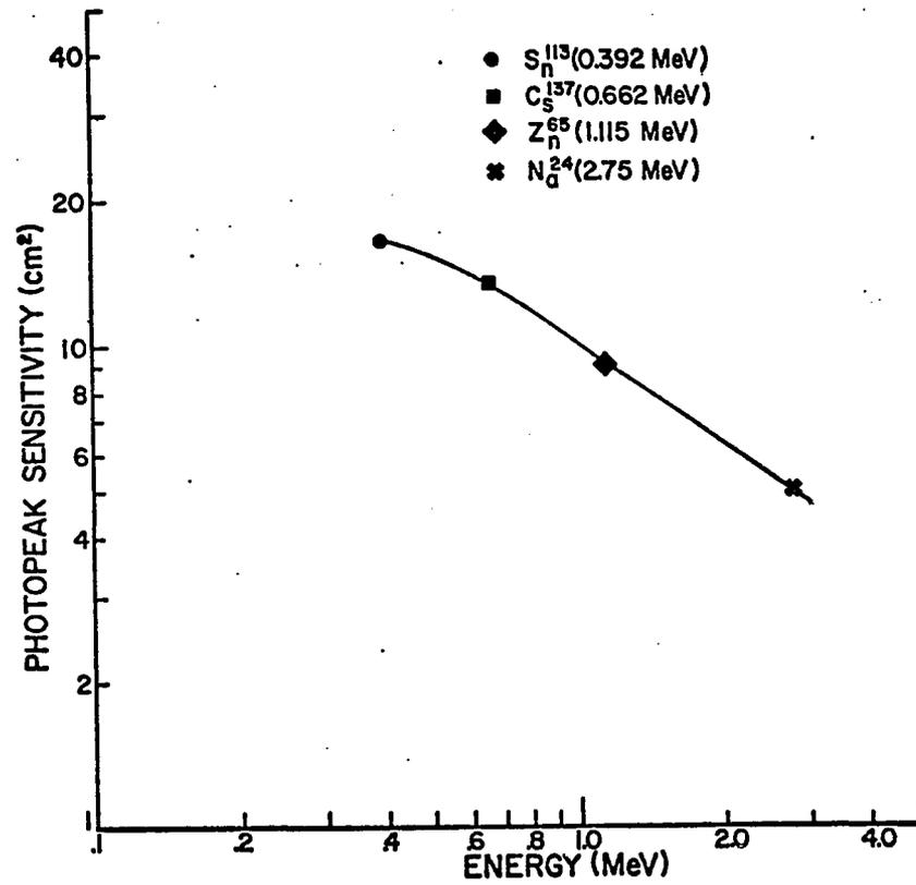
Figure II-2. Energy dependence of the detector sensitivity (cm<sup>2</sup>) for an axial parallel beam for four line sources.
