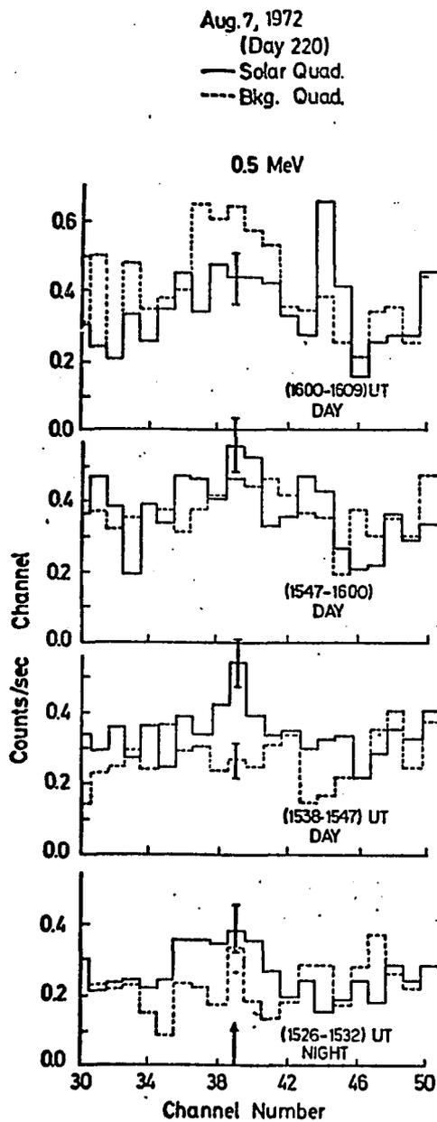
Figure IV-13. The gamma-ray pulse height spectrum for the energy region 435 - 610 keV on August 7, 1972. The  $H_{\alpha}$  flare began about 1500 UT during satellite night. Satellite sunrise occurred at 1538 UT.
