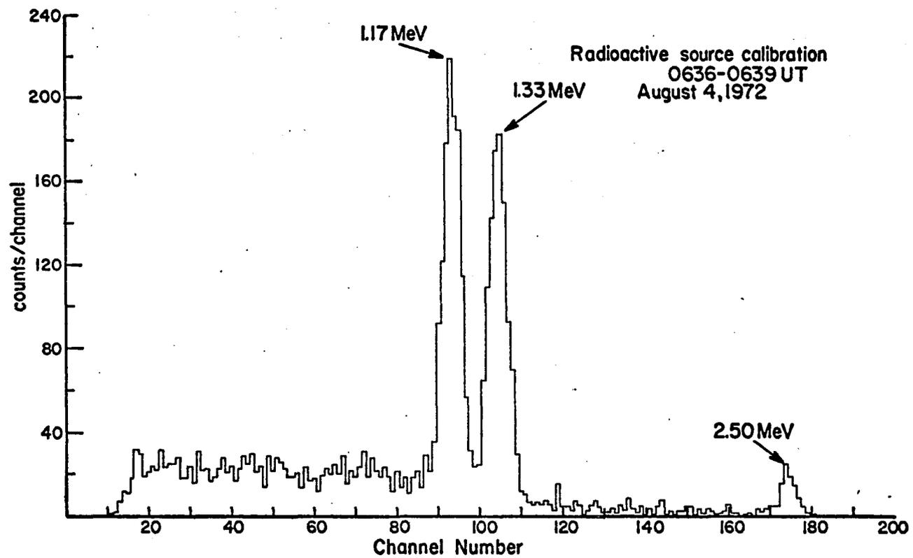
Figure II-5. Sample  $\text{Co}^{60}$  calibration spectrum obtained in orbit.
