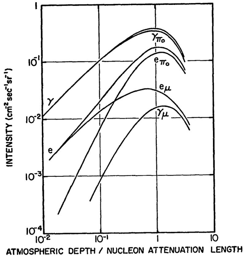
Figure A-2. Intensities of electrons ( $e$ ) and gamma rays ( $\gamma$ ) of energies above 100 MeV versus atmospheric depth, in units of the nucleon attenuation length,  $110 \text{ g} \cdot \text{cm}^{-2}$ . The contributions of  $\pi^0 - 2\gamma$  decays ( $\gamma_{\pi^0}$ ,  $e_{\pi^0}$ ) and  $\pi - \mu - e$  decays ( $\gamma_{\mu}$ ,  $e_{\mu}$ ) to gamma rays and electrons are shown separately. (Hayakawa, 1969).
