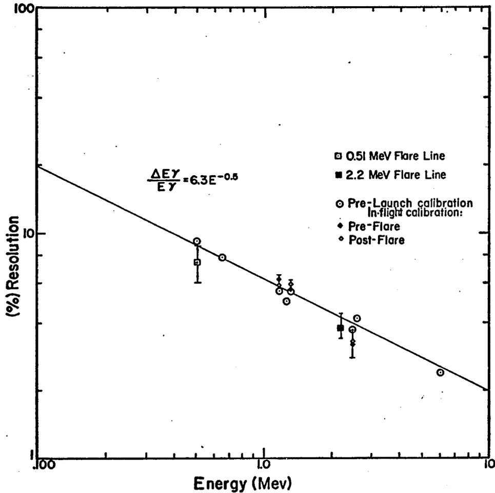
Figure IV-14. The dependence of energy resolution on energy for the UNH detector as obtained from prelaunch calibration data (○). Pre-flare (◆) and post-flare (◇) values for resolution come from  $\text{Co}^{60}$  calibration spectra. The measured line widths for the 0.51 and 2.2 MeV flare lines are also shown.
