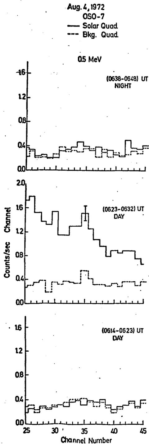
Figure IV-12. The gamma-ray pulse height spectrum for the energy region 435 - 615 keV on August 4, 1972. The  $H_{\alpha}$  flare began about 0621 UT and the satellite was occulted by the Earth at about 0633 UT.
