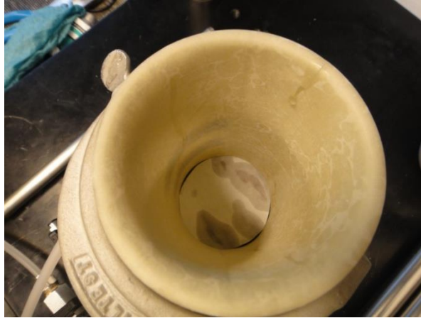
Figure F-116. Installed porous stone with filter paper on top
