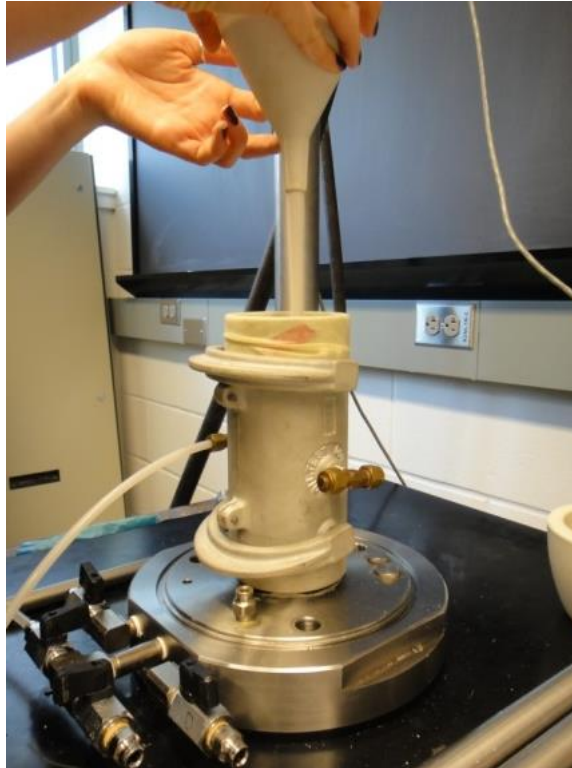
Figure 21 Dry pluviation of Ottawa F75 sand
