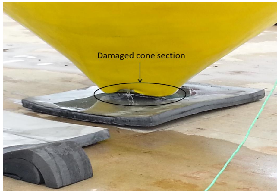
Figure 55: Damaged cone section on the bottom of the buoy after being pivoted on.
