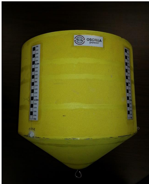
Figure 45: Froude scaled model buoy of full scale design constructed by Oscilla Power and used for physical model testing.
