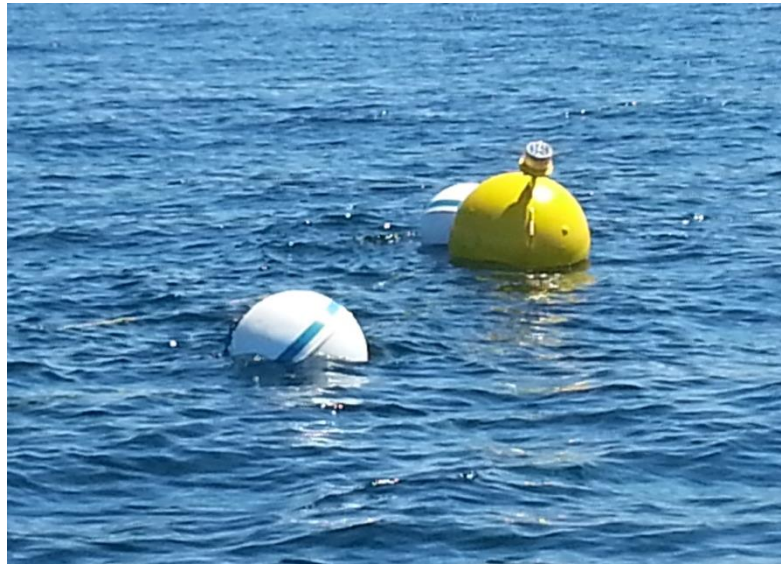
Figure 54: Temporary floats terminating each of the three mooring lines connected together. These floats were removed and replaced with the full scale buoy for testing.
