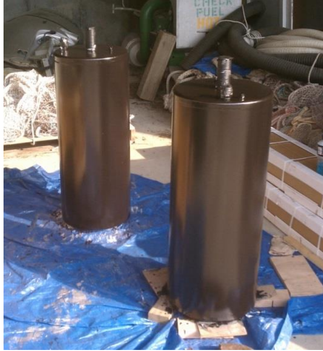
Figure 28: Final result of preventative paint coatings.
