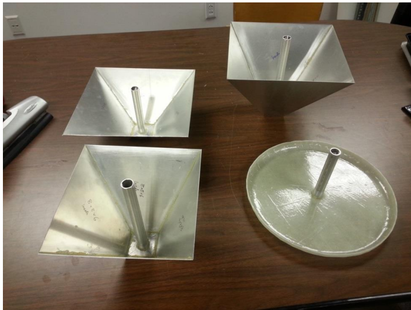
Figure 35: Model heave plates to be used in tank testing. The 10x10x4 model is shown in top left; the 10x10x7 is shown in top right; the 8x8x6 is shown in bottom left, and the circular model is shown in bottom right.
