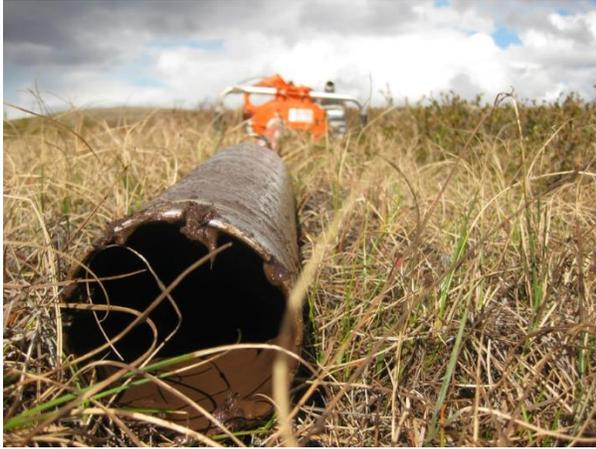
Gas-powered auger with a peat corer barrel attached (Photo: Adam Wlostowski, Penn State U.)
